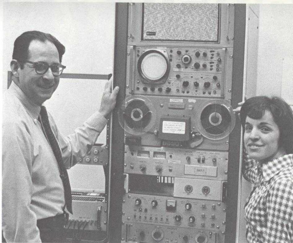
Drs. Campanella and Robinson display the baseband processing branch's analog-digital/digital-analog data link. The device converts analog signals like speech or television to digital form for Fast Fourier Transform (FFT) computer analysis. It can also "play back" by reconverting digital data to analog signals for subjective evaluation.
