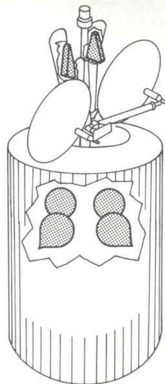
A simplified drawing of INTELSAT IV showing the four fuel tanks in the spinning drum and the two nutation dampers on the despun platform.
