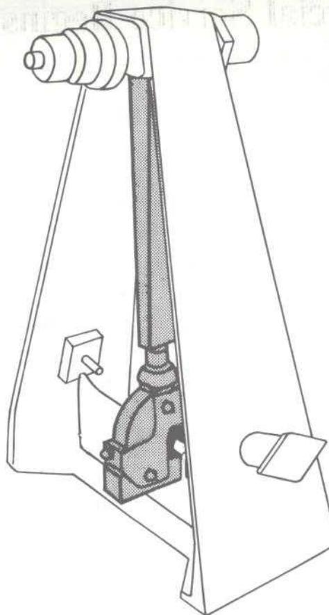
An actual nutation damper for INTELSAT IV. The dark area is the pendulum arm. The device is open, just as you see it here.
