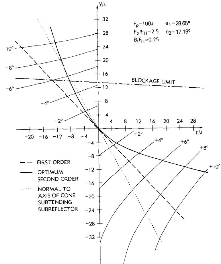
Figure 7. Optimum Locus and Constant Beam Direction Loci for a Few Angles (Both Approximations)
