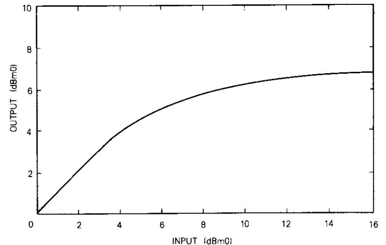
Figure 16. MUX Transmit Channel Limiter Characteristics
