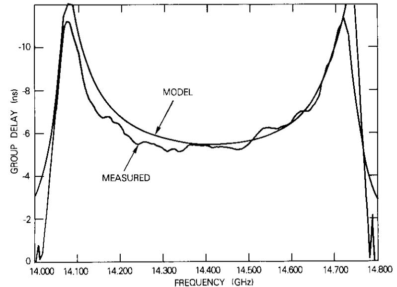
Figure 9. Measured Time Delay of a Time-Delay Filter
