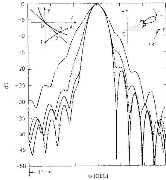
Figure 10. The Pattern in the Plane of Symmetry for the Feed at Several Positions, Scan Angle =  $+4^\circ$
