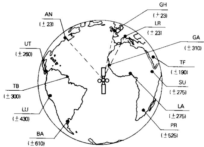
Figure 6. Synchronization Accuracy of Open-Loop TDMA System (Ranging Stations AN, GH, and LR)
