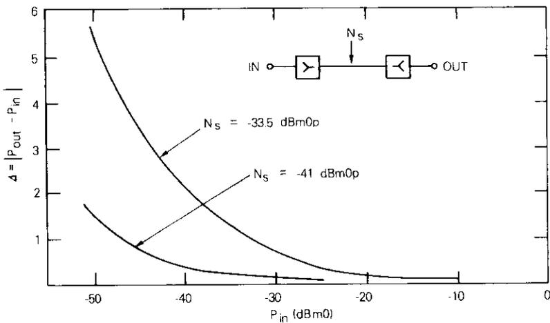
Figure 7. Tracking Error in the Presence of System Noise
