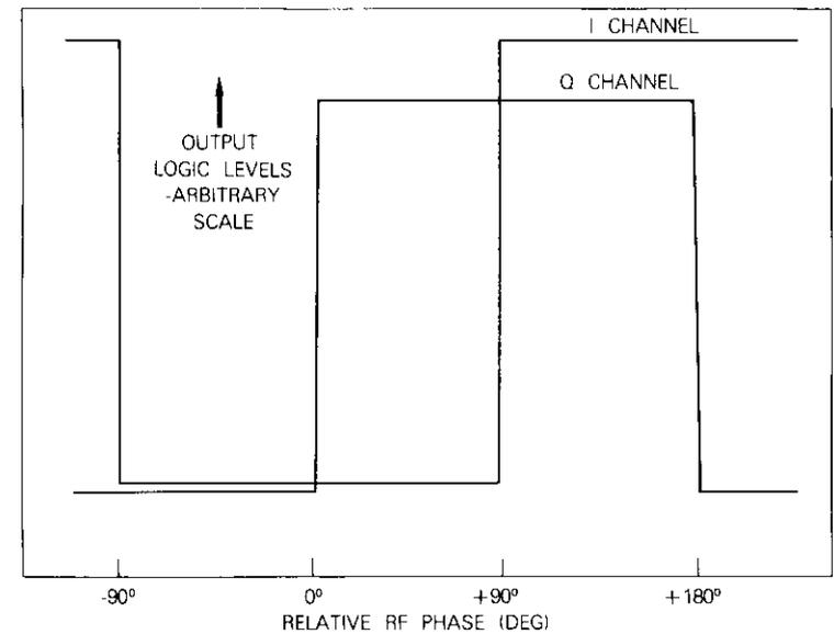
Figure 14. Measured Phase Response of the QPSK Demodulator Showing Output Logic Levels
