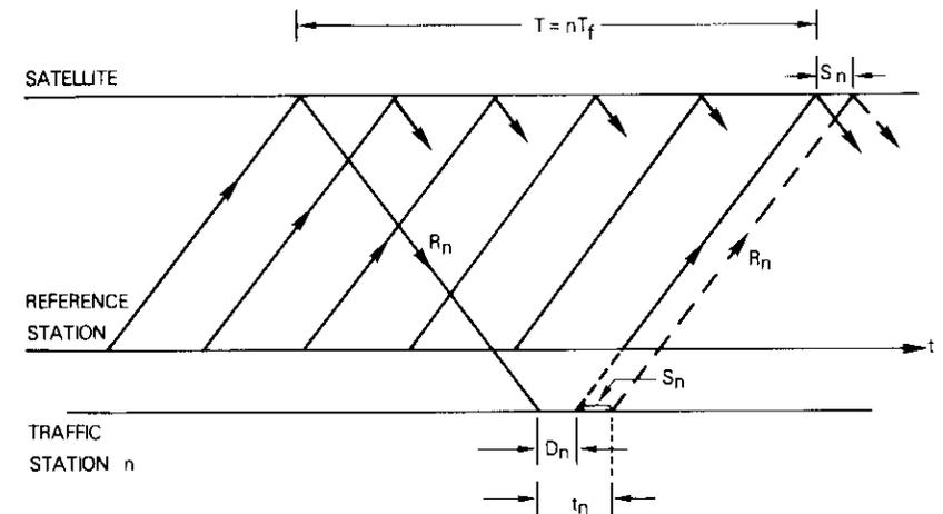
Figure 1. Burst Transmission Timing Diagram
