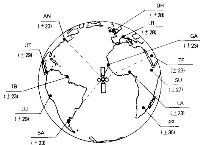
Figure 5. Synchronization Accuracy of Open-Loop TDMA System (Ranging Stations AN, BA, and TF)
