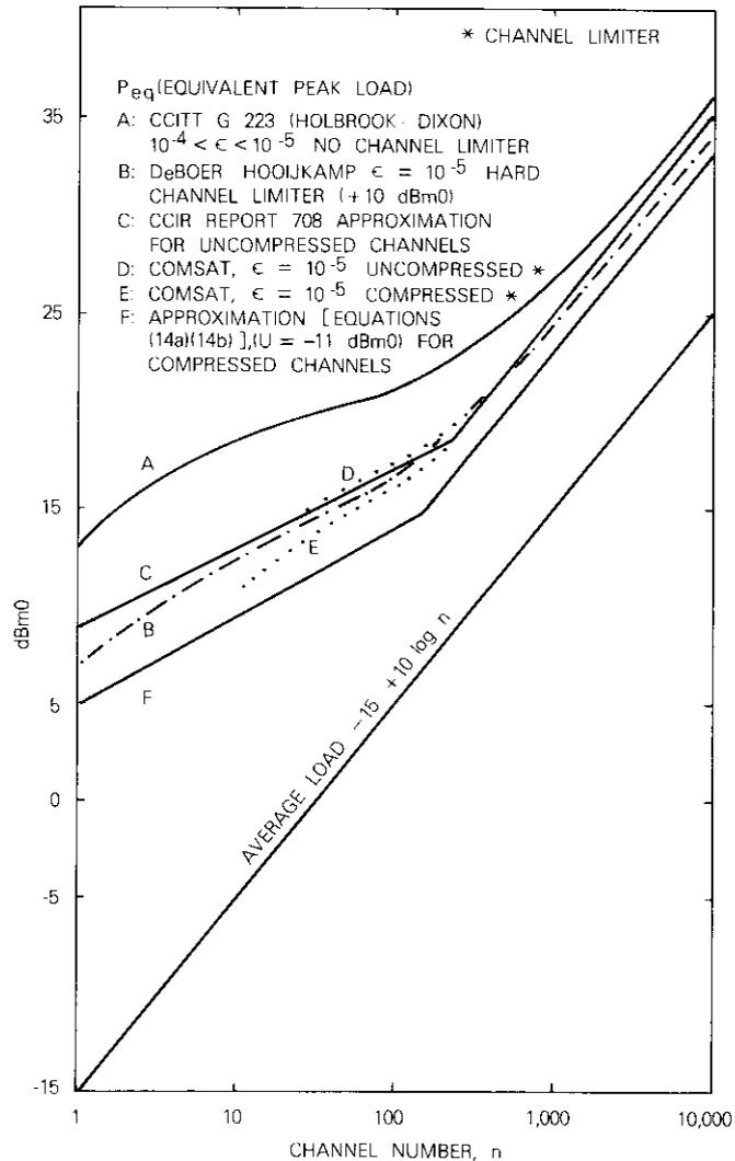
Figure 15. Multichannel Equivalent Peak Load
