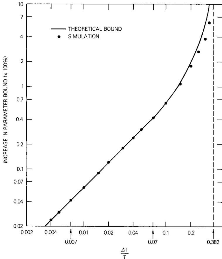
Figure 4. Increase in Parameter Bound for Delayed Clock Correction
