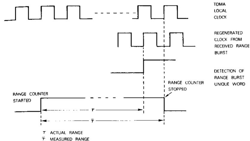
Figure 3. Range Counter Clock Resolution Error
