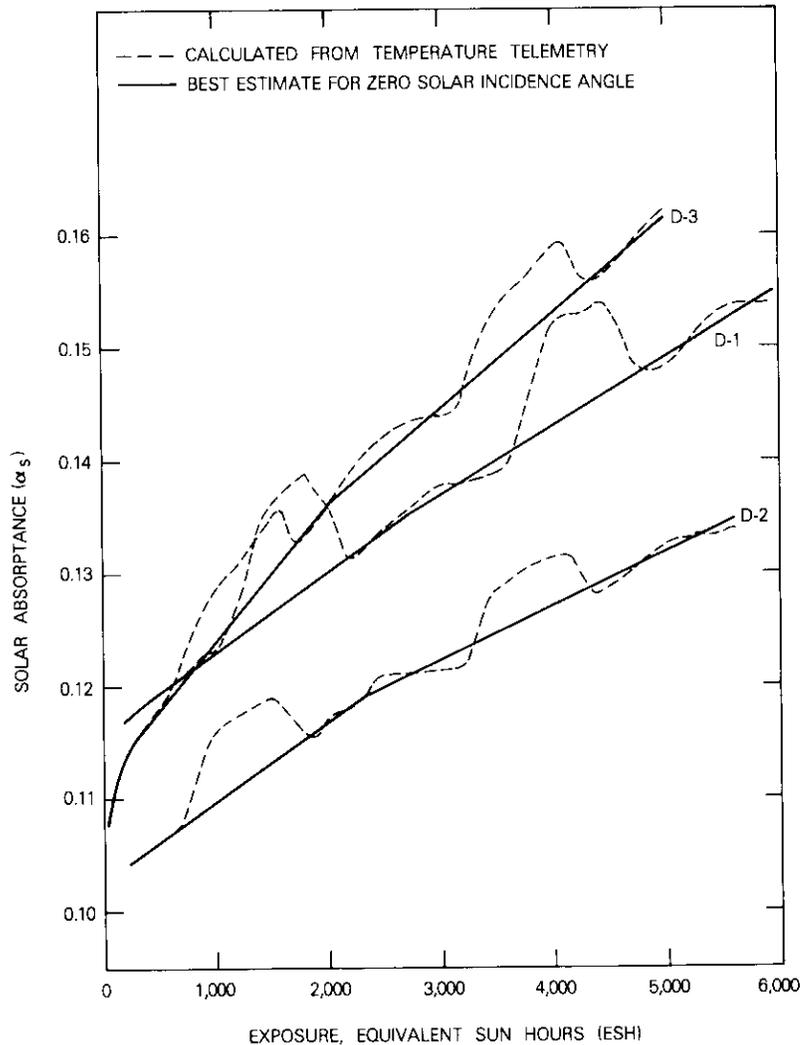
Figure 9. Solar Absorptance Histories of 28-GHz Beacon Radiators on COMSTAR D-1, D-2, and D-3
