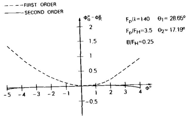
Figure 5. Accuracy Comparison for the Constant Beam Scan Angle Loci for Both Approximations,  $F_p = 140\lambda$
