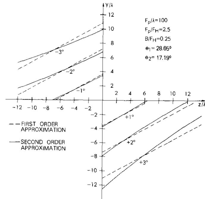
Figure 4. Constant Beam Direction Loci for  $F_p = 100\lambda$
