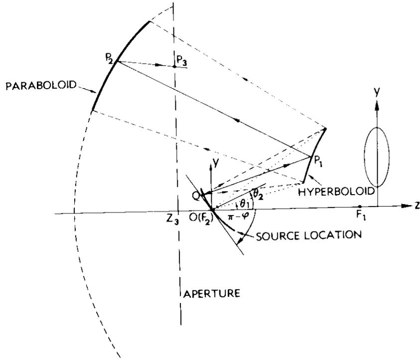
Figure 1. Antenna Geometry
