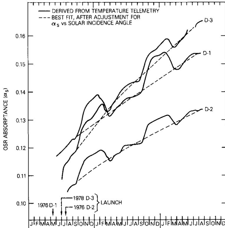
Figure 4. 28-GHz Beacon OSR Absorptance vs Time on COMSTAR D-1, D-2, and D-3
