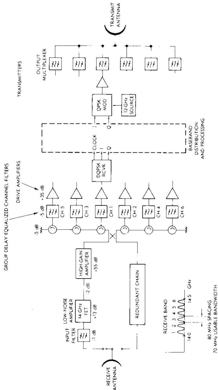
Figure 1. Block Diagram of a Regenerative Transponder
