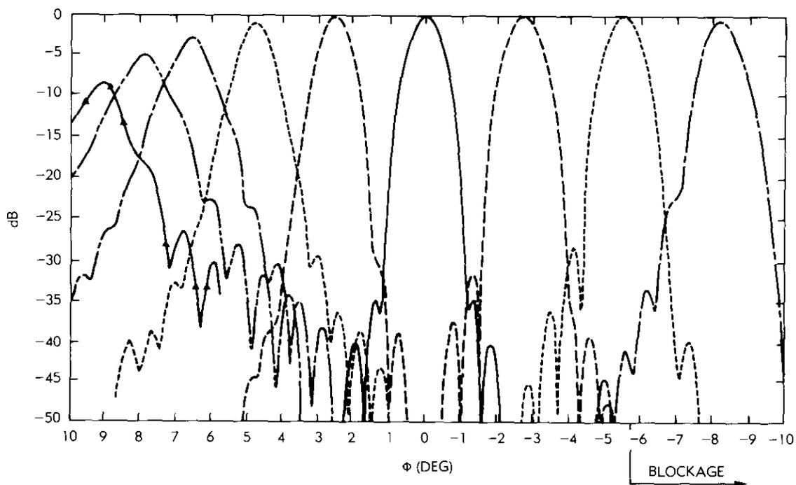
Figure 14. Scanned Beams for Offset Cassegrain with Feed Displaced Along Normal to Axis of Cone Subtending the Subreflector ( $\theta_1 + \pi/2$ )
