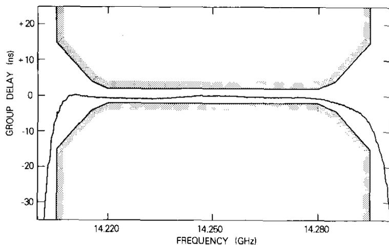
Figure 3. Measured Group Delay for the Channel Filter
