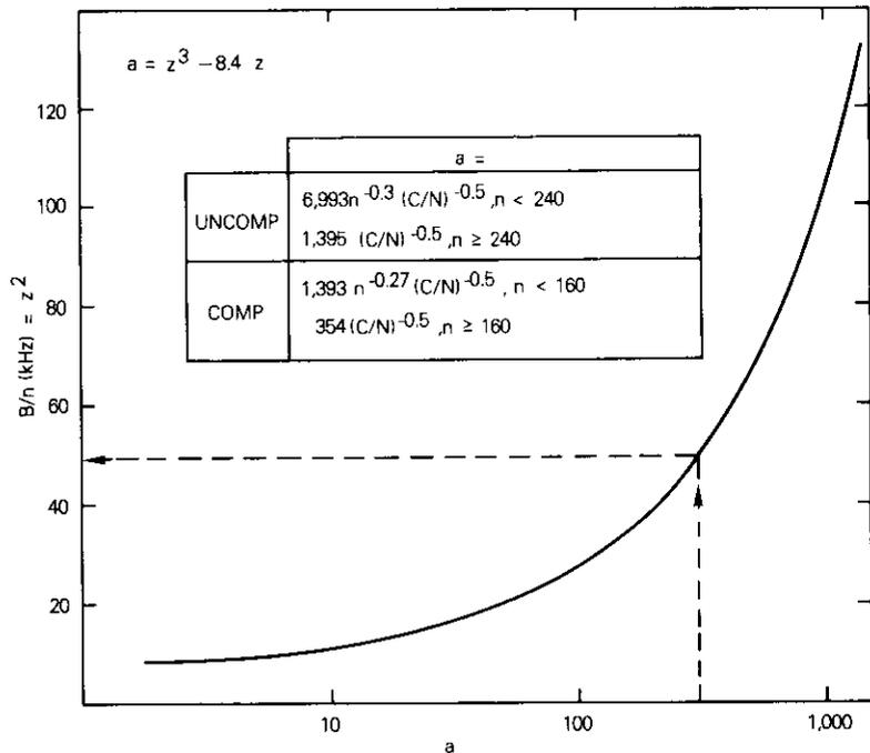
Figure 25. Graphical Solution of the FM Equation
