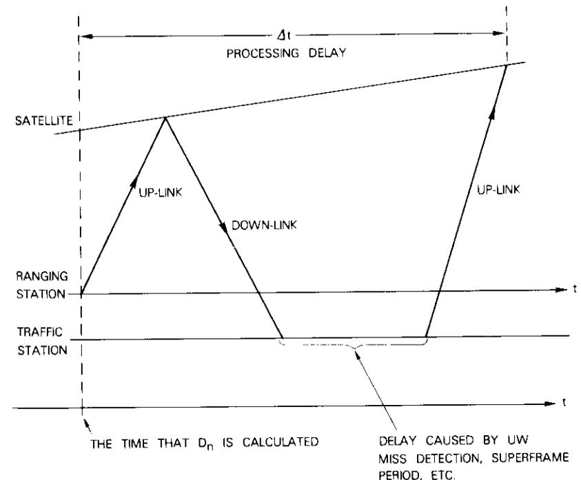
Figure 4. Processing Delay
