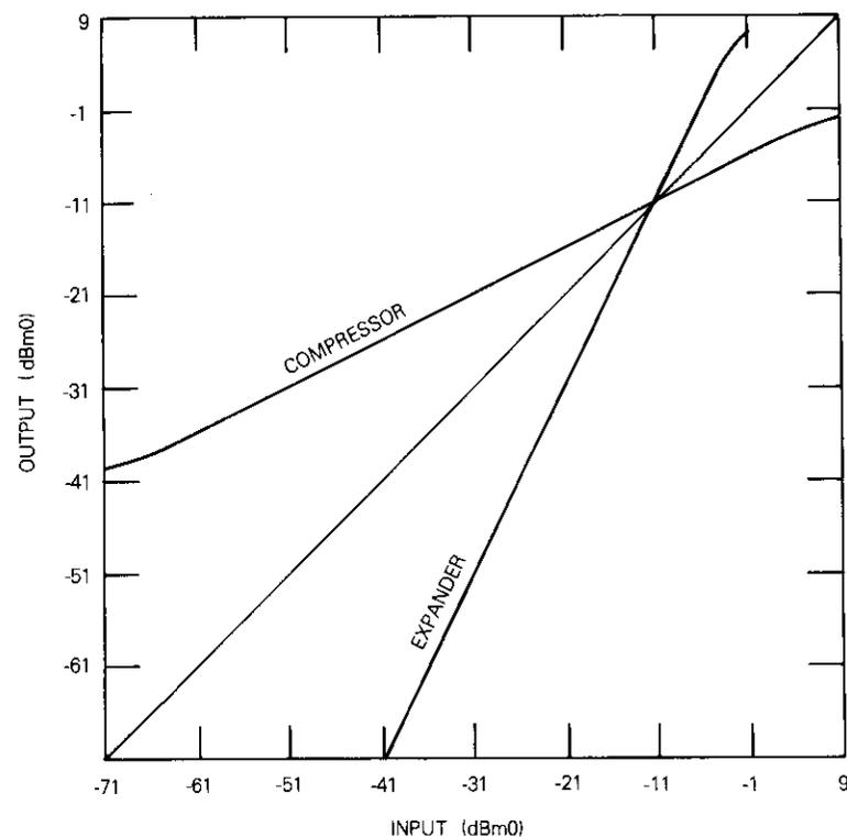
Figure 5. Compressor and Expander Characteristics
