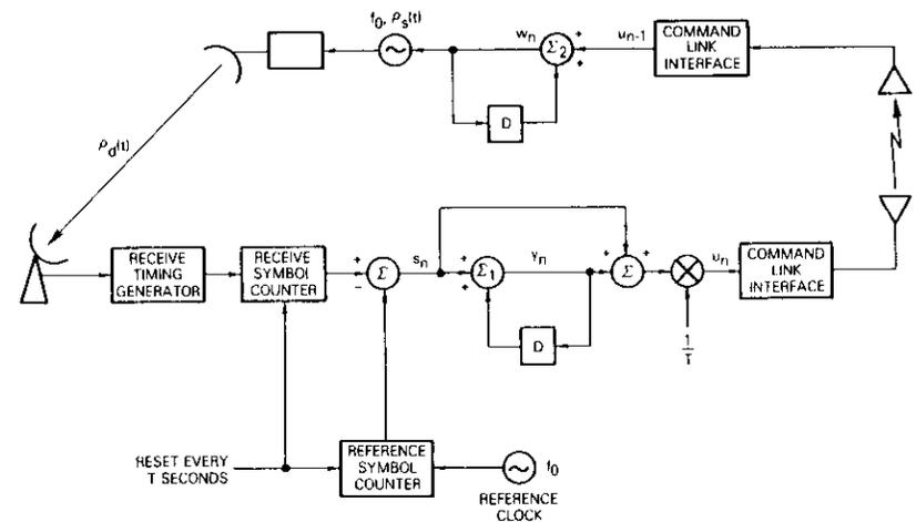
Figure 5. Onboard Clock Correction Diagram for Baseband Processing Satellite
