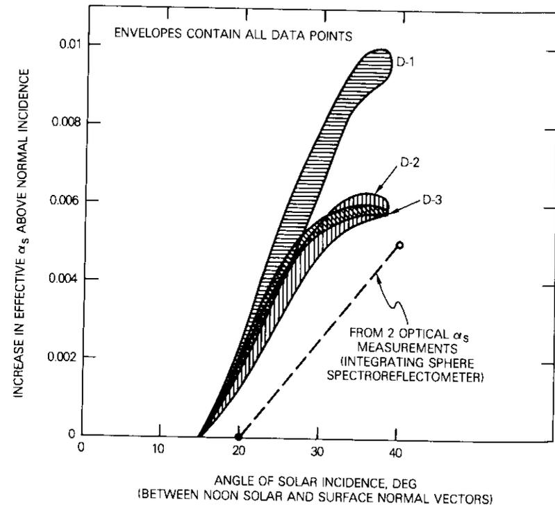
Figure 6. Effective Absorptance as a Function of Noon Angle of Solar Incidence on 28-GHz Beacon Radiator
