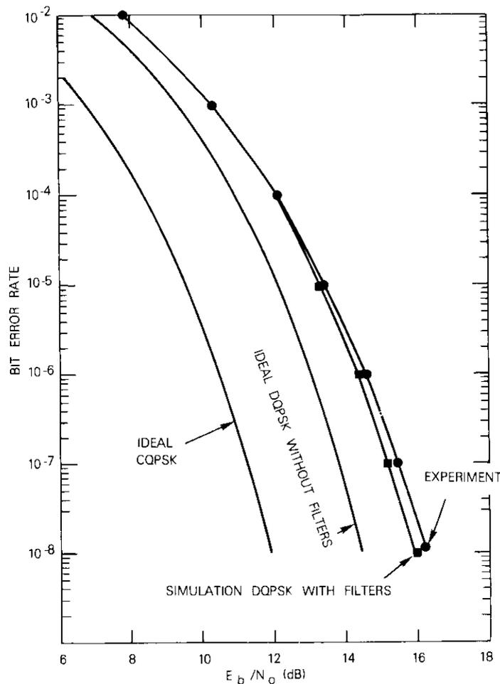
Figure 18. Measured Bit-Error Rate of the DQPSK Receiver
