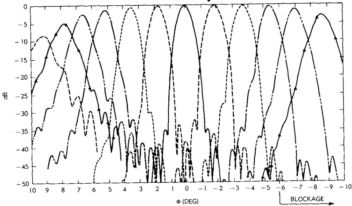
Figure 13. Scanned Beams for Offset Cassegrain with Feed Displaced Along First-Order Approximation Optimum Locus (straight line)
