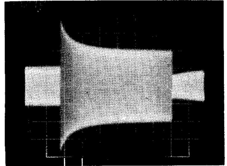
Figure 8. Compressor Attack Response
