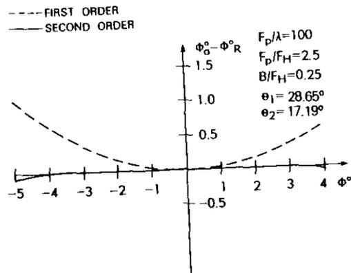
Figure 6. Accuracy Comparison for the Constant Beam Scan Angle Loci for Both Approximations,  $F_p = 100\lambda$
