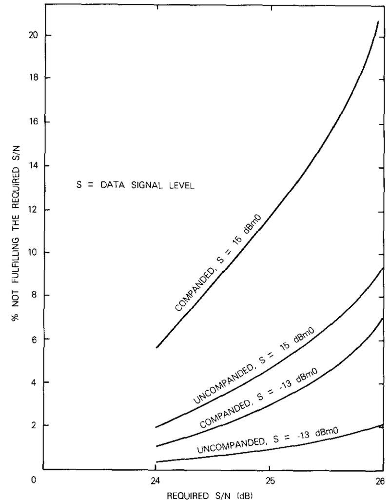
Figure 29. Probability of Not Fulfilling the S/N Requirements
