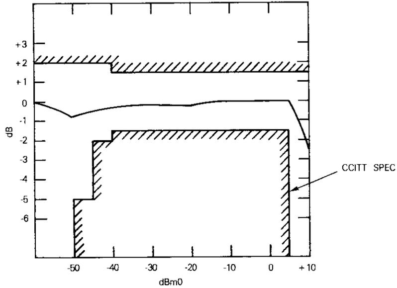
Figure 6. Compressor Tracking Curve
