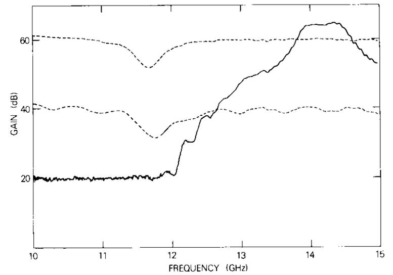
Figure 6. Measured Out-of-Band Response of the 14-GHz FET Amplifier
