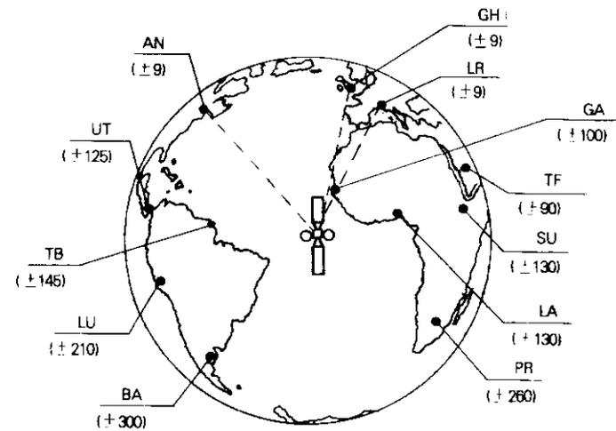
Figure 8. Synchronization Accuracy of the Improved Open-Loop TDMA System (Ranging Stations AN, GH, and LR)
