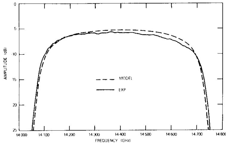
Figure 8. Measured Transmission Response of a Time-Delay Filter
