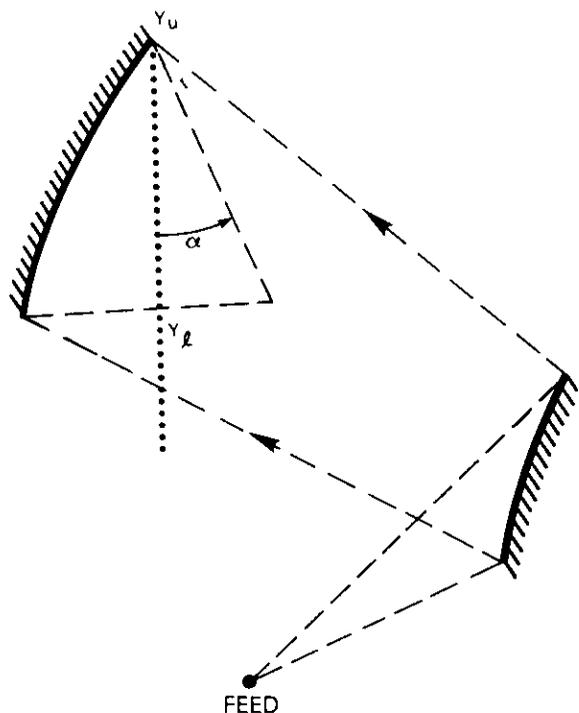
Figure 2. Definition of the Beam Scan Angle
