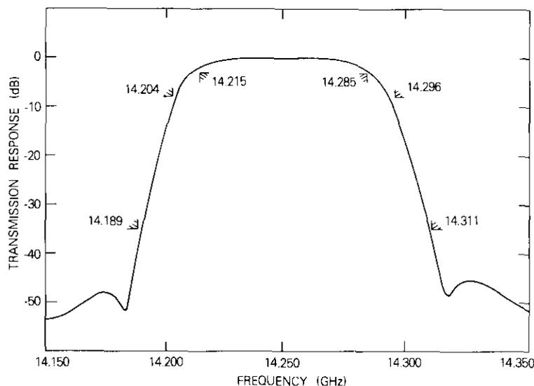
Figure 2. Measured Transmission Response of the Channel Filter
