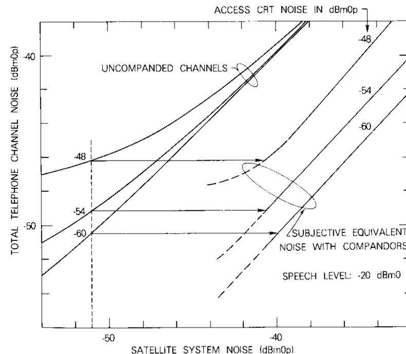
Figure 14. Channel Noise vs Satellite System Noise
