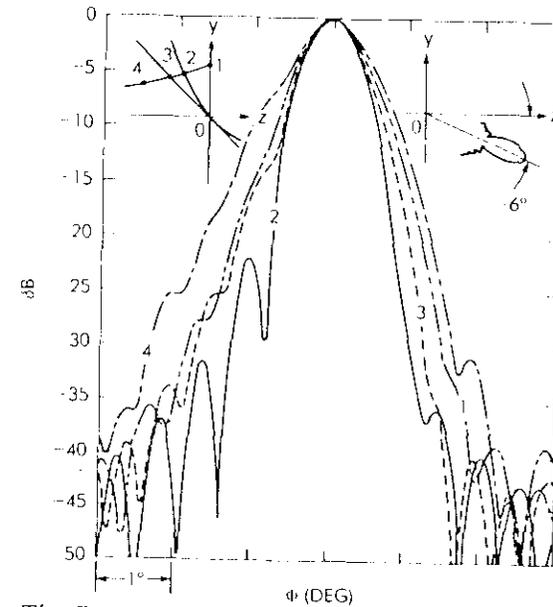
Figure 8. The Pattern in the Plane of Symmetry for the Feed at Several Positions, Scan Angle =  $-6^\circ$
