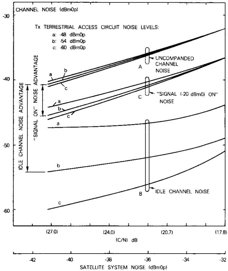
Figure 12. Channel Noise vs Satellite System Noise
