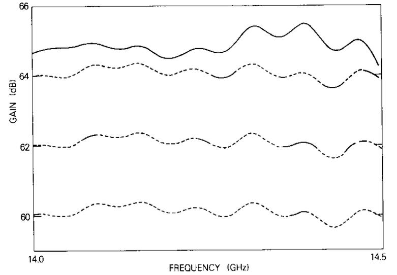
Figure 5. Measured In-Band Response of the 14-GHz FET Amplifier
