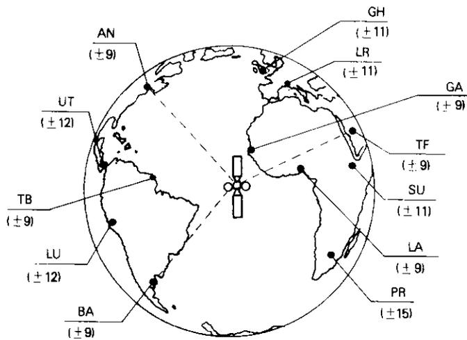
Figure 7. Synchronization Accuracy of the Improved Open-Loop TDMA System (Ranging Stations AN, BA, and TF)
