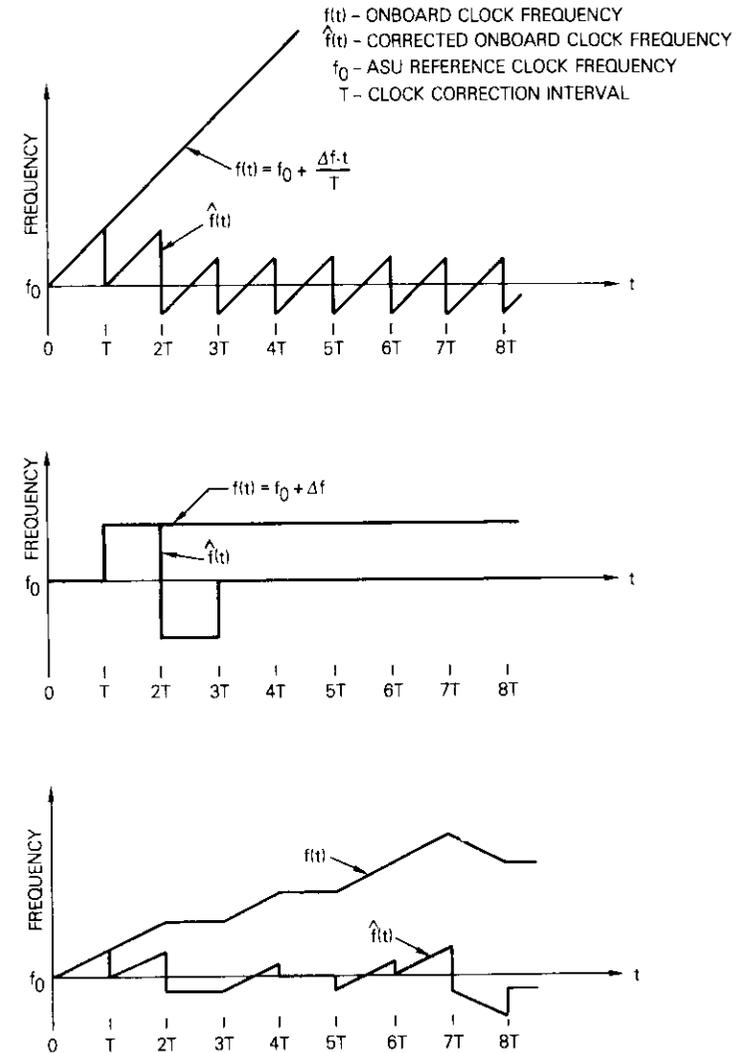
Figure 3. Examples of Clock Correction
