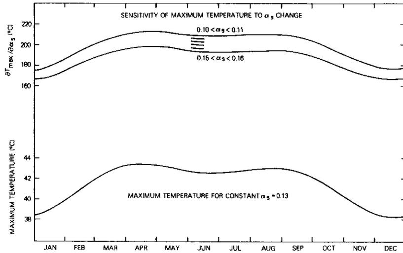
Figure 2. Predicted Maximum Diurnal Temperature Characteristics of 28-GHz Beacon on COMSTAR D-2 and D-3: 32 W Dissipation
