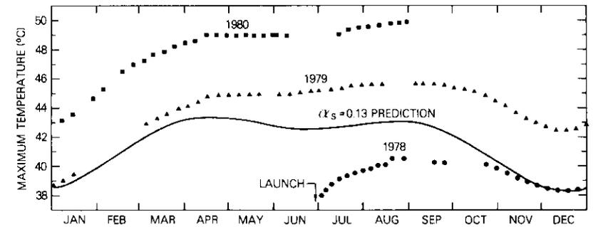
Figure 3. 28-GHz Beacon on COMSTAR D-3: History of Telemetered Maximum Daily Temperature and Predicted Maximum Temperature for  $\alpha_s = 0.13$
