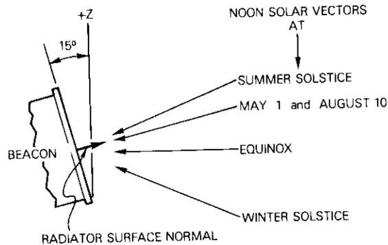
Figure 1. Beacon-on-COMSTAR Geometry
