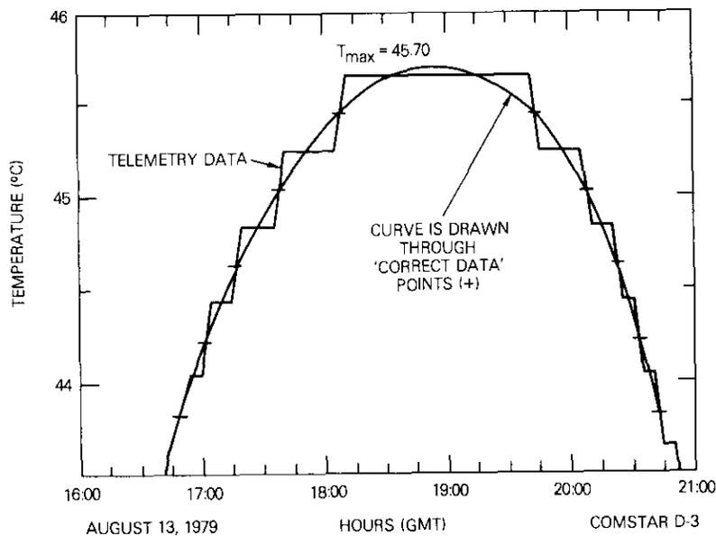
Figure 8. Example of Temperature Telemetry Display and Graphical Procedure for Obtaining Maximum Temperature
