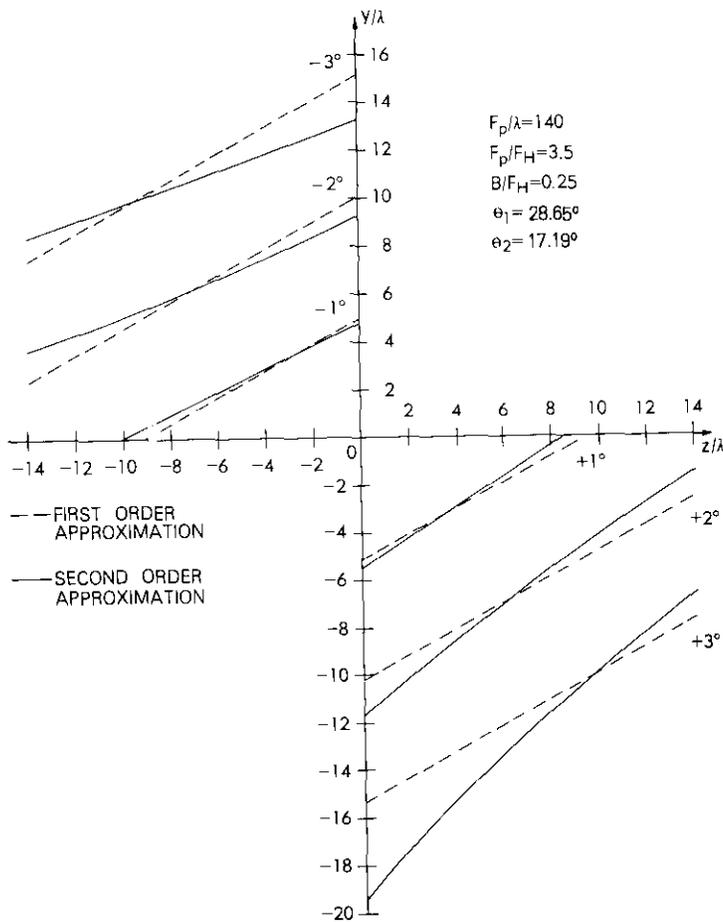
Figure 3. Constant Beam Direction Loci for  $F_p = 140\lambda$
