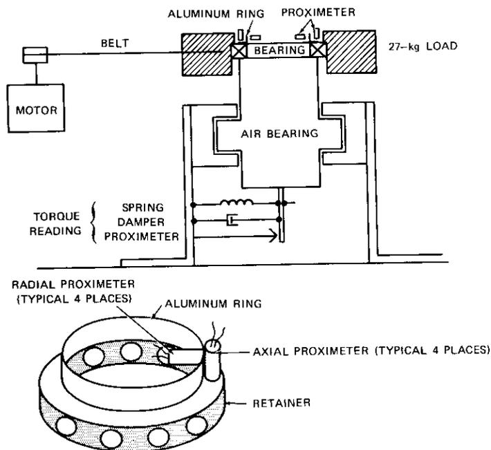
Figure 5. Bearing Test Setup
