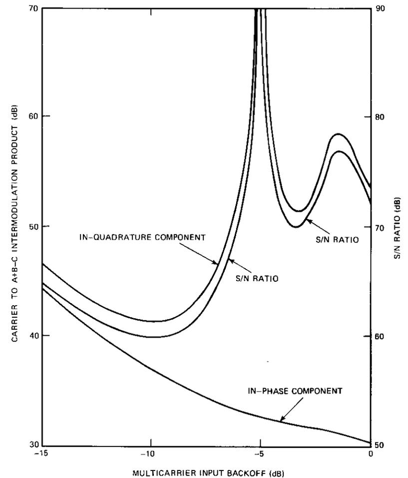
Figure 13. Carrier-to-Intermodulation Ratio and S/N vs Multicarrier Input Backoff
