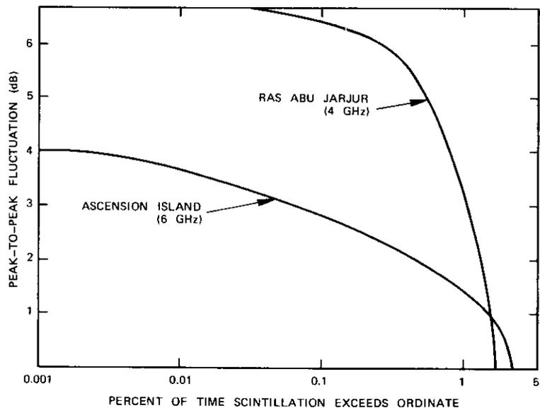
Figure 3. Cumulative Amplitude Distributions at Ascension Island (6 GHz) and Ras Abu Jarjur (4 GHz)
