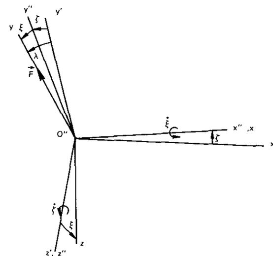
Figure 3. Nomenclature for Thrust Vector Angular Misalignment
