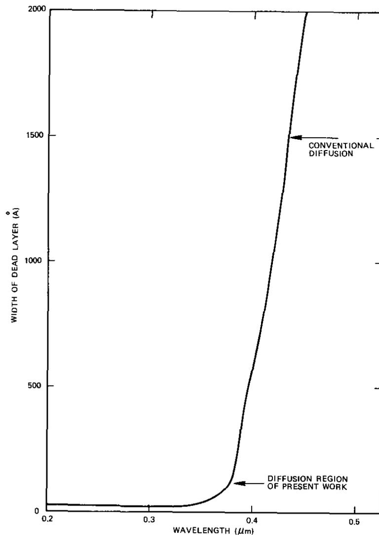
Figure 7. Maximum Dead Layer Thickness as a Function of Cutoff Wavelength for 71-percent Response
