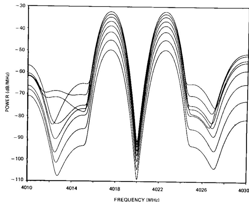
Figure 11. RF Intermodulation Power Spectral Density Generated by a TV Carrier (spreading only) and Two Program Channels
