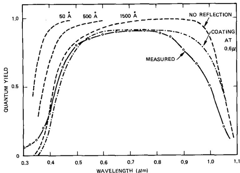
Figure 6. Plot of Calculated Short Wavelength Response Using Dead Layer Model
