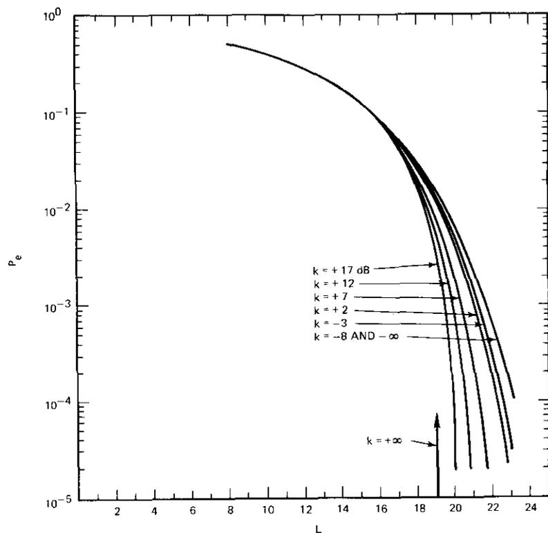
Figure 5c. Error Probabilities of 16-Phase PSK in the Presence of Gaussian Noise and Three Cochannel Interferences ( $H = 3, 16\phi$ )
