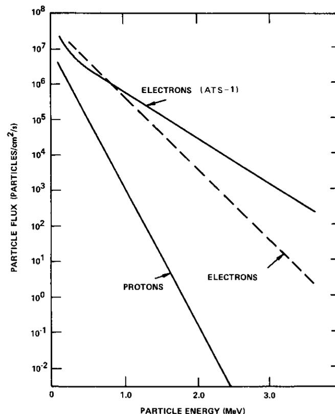
Figure 1. *Time-Averaged Trapped Flux at Synchronous Altitude*
