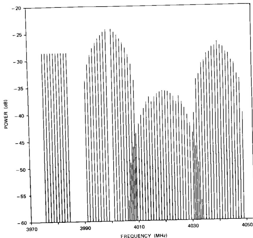
Figure 6. 3rd-Order RF Intermodulation Products Generated by 10 Equal Carriers and a Single Carrier
