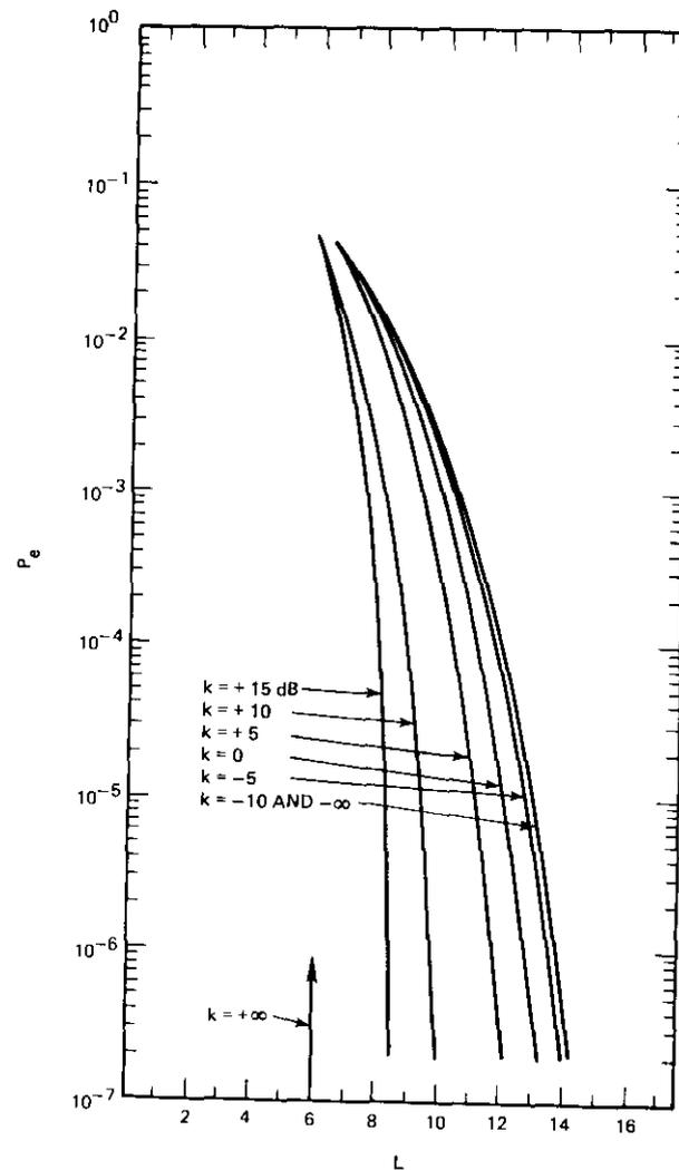
Figure 3b. Error Probabilities of 4-Phase PSK in the Presence of Gaussian Noise and Two Cochannel Interferences ( $H = 2, 4\phi$ )
