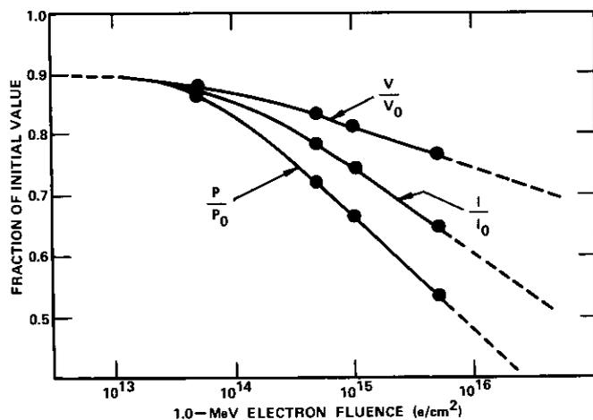
Figure 5. Silicon Solar Cell Output Degradation
