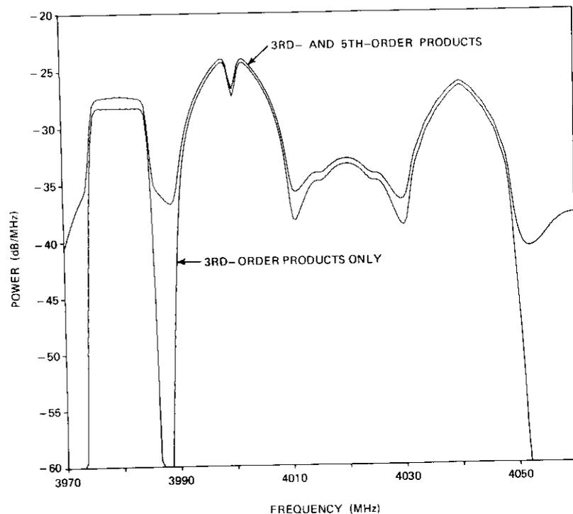
Figure 8. RF Intermodulation Power Spectral Density Generated by 10 Equal Carriers and a Single Carrier
