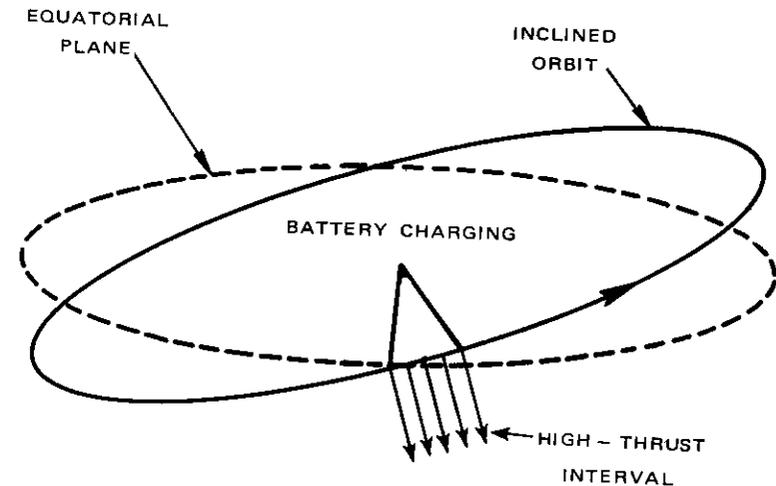
Figure 3. Thrust Program for North-South Stationkeeping with Battery-Powered Electric Propulsion
