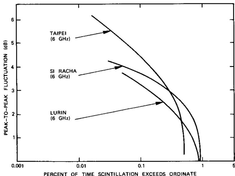
Figure 8. Cumulative Amplitude Distributions at Lurin (6 GHz), Taipei (6 GHz), and Si Racha (6 GHz)
