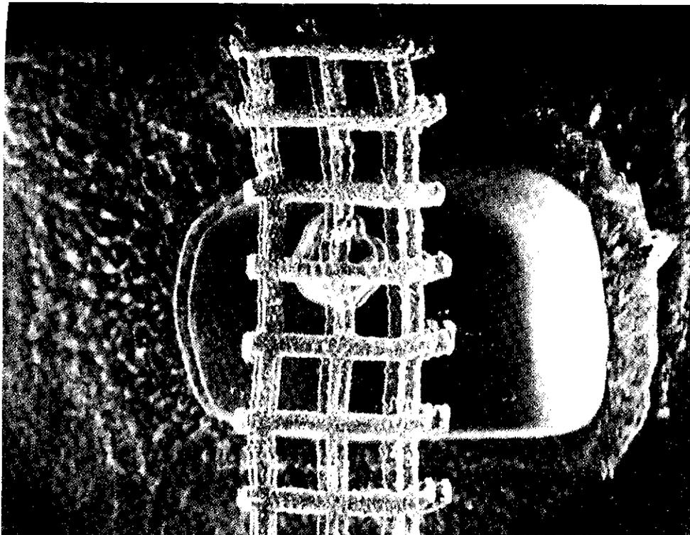
PLATE II. *Stereoscopic SE Image of a Germanium Tunnel Diode (top view)*
