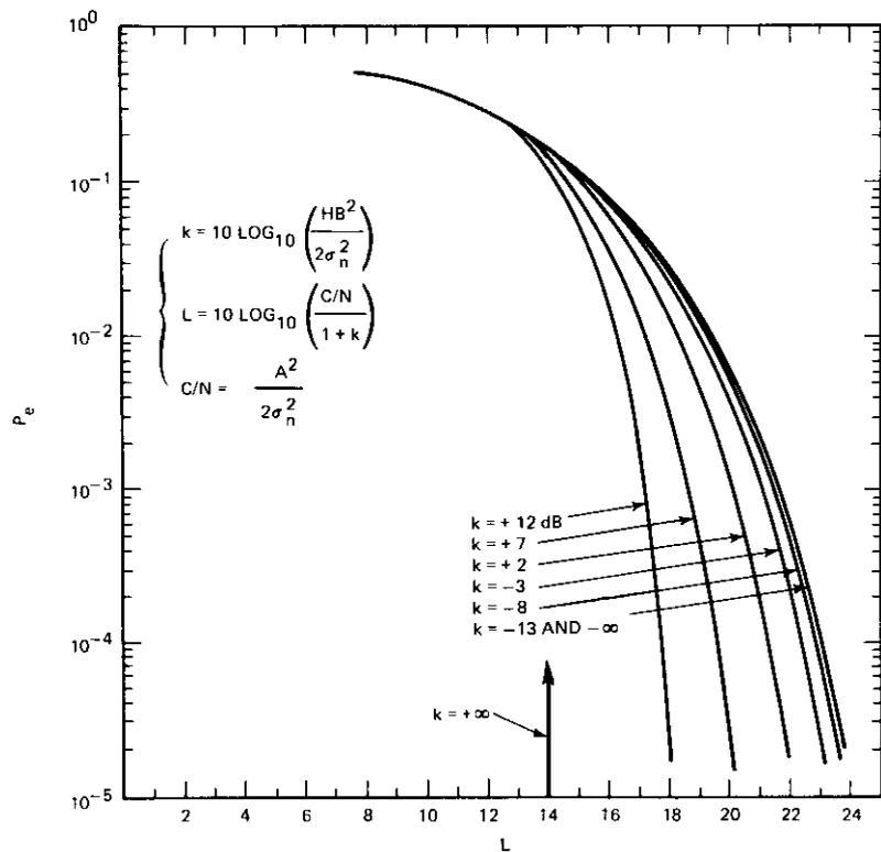
Figure 5a. Error Probabilities of 16-Phase PSK in the Presence of Gaussian Noise and One Cochannel Interference ( $H = 1, 16\phi$ )
