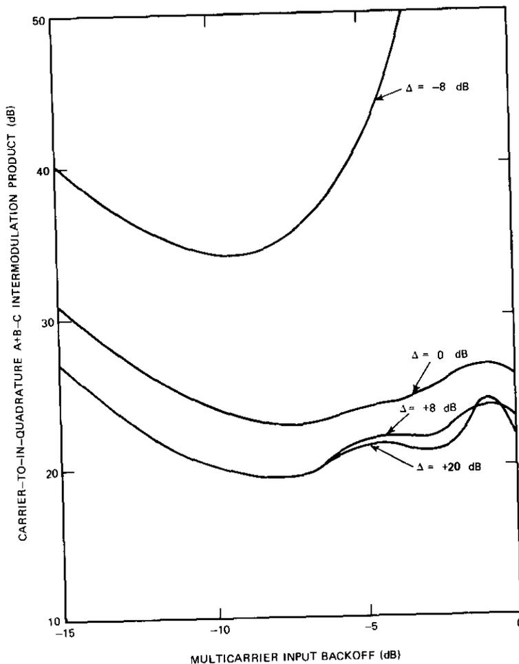
Figure 16. Carrier-to-In-Quadrature Intermodulation Ratio vs Multicarrier Input Backoff
