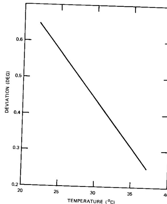
Figure 2. Peak Platform Deviation vs Temperature
