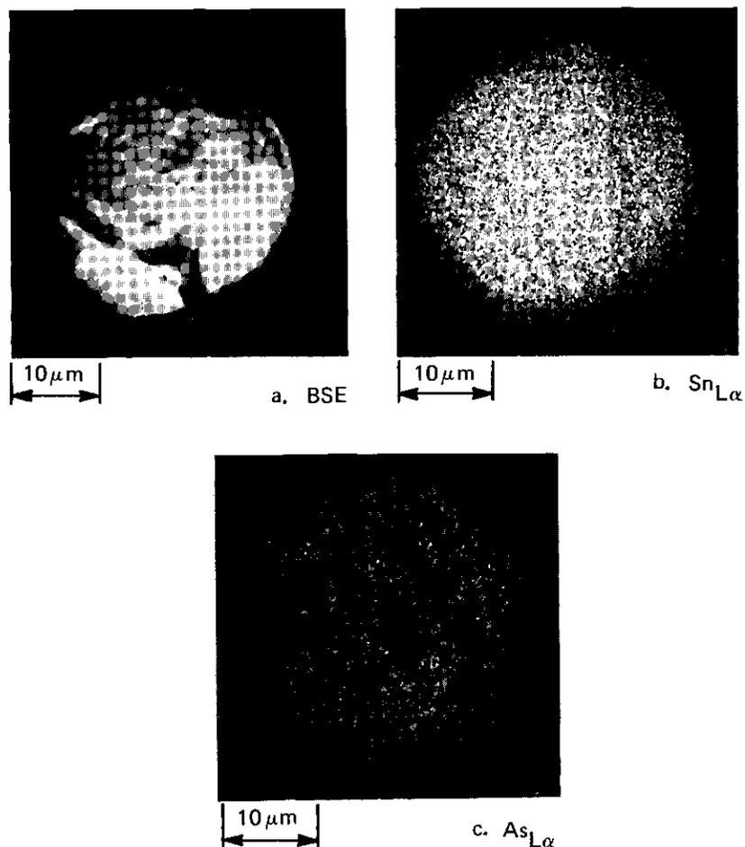
Figure 2. Sn-Doped As Ball Before Alloying
