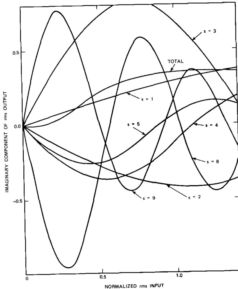
Figure 4. Bessel Function Expansion of the Imaginary Component of the Single-Carrier Transfer Function
