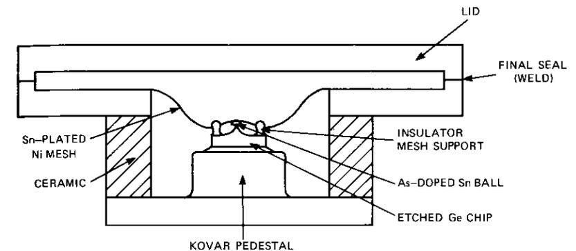
Figure 1. Schematic Cross-section of Ball Alloy Ge Tunnel Diode
