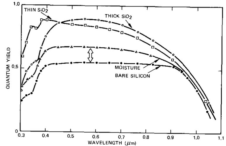
Figure 5. Quantum Yield per Incident Photon for Two Thicknesses of Thermal  $\text{SiO}_2$  and Bare Silicon Surface in Dry and Moist Ambients
