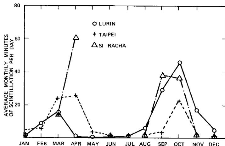
Figure 11. Seasonal Variation of Ionospheric Scintillation Greater than 0.5 dB at Lurin, Taipei, and Si Racha
