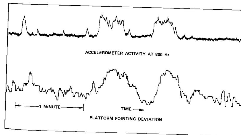
Figure 3. 800-Hz Accelerometer Noise Platform Pointing Deviation
