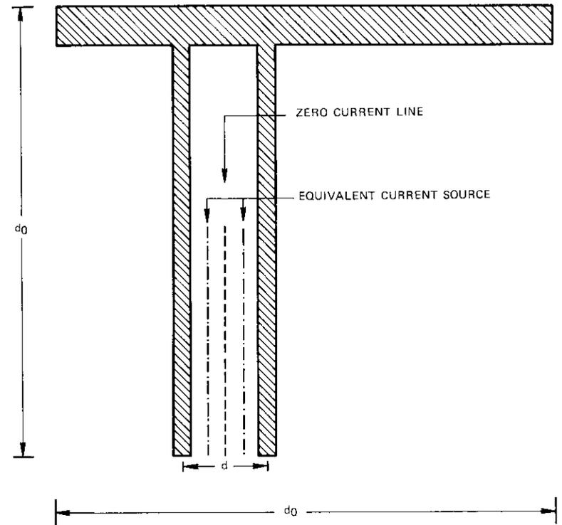
Figure 1. Simple Illustrative Aid for Calculation of Series Resistance as a Function of Grid Spacing
