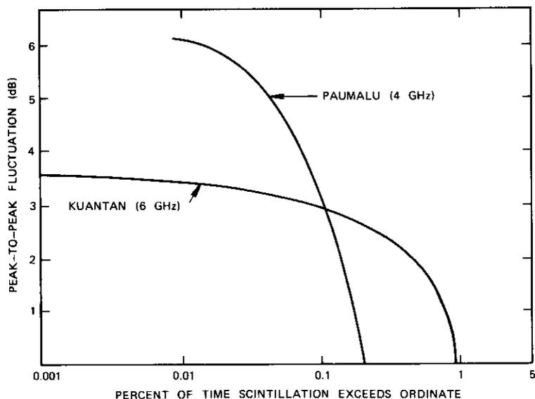
Figure 7. Cumulative Amplitude Distributions at Kuantan (6 GHz) and Paumalu (4 GHz)
