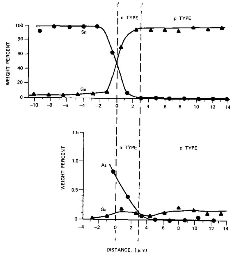
Figure 6. Sn, As, Ge, and Ga Distributions Measured in Ball Alloy Diode Cross-section
