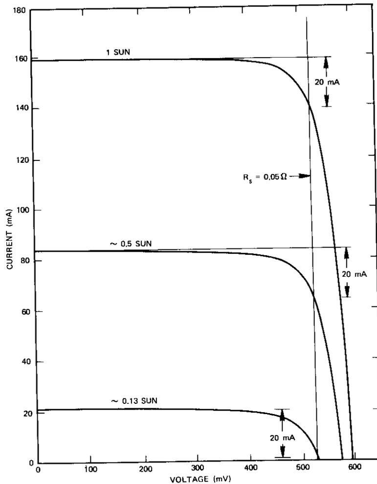
Figure 11. Measurement of Total Series Resistance under AM0 Illumination Using Neutral Density Filters
