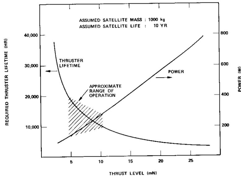
Figure 1. Tradeoff Between Electric Thruster Lifetime and Required Power
