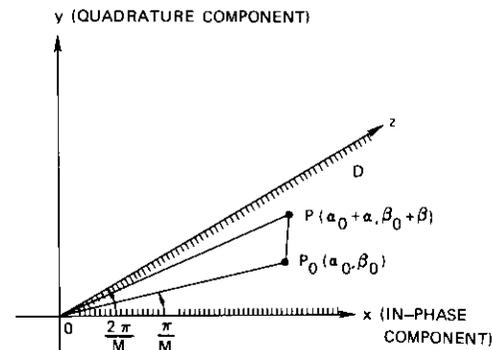
Figure 2. Signal Space of PSK Systems
