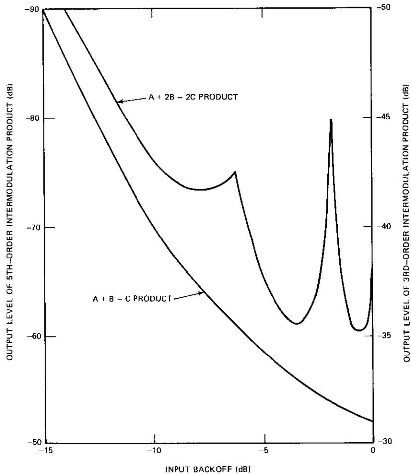
Figure 12. Intermodulation Product Level as a Function of Input Backoff
