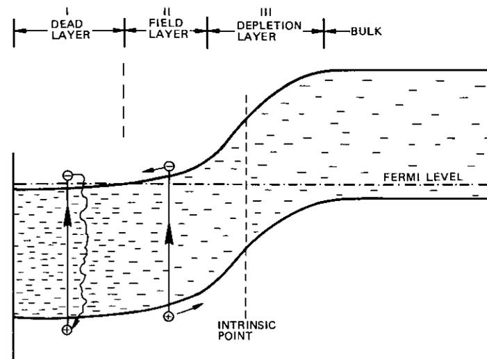
Figure 4. Energy Band Diagram for  $n^+p$  Junction
