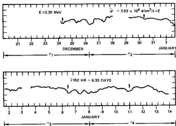
Figure 2. Time Variation of Electron Flux at Synchronous Altitude
