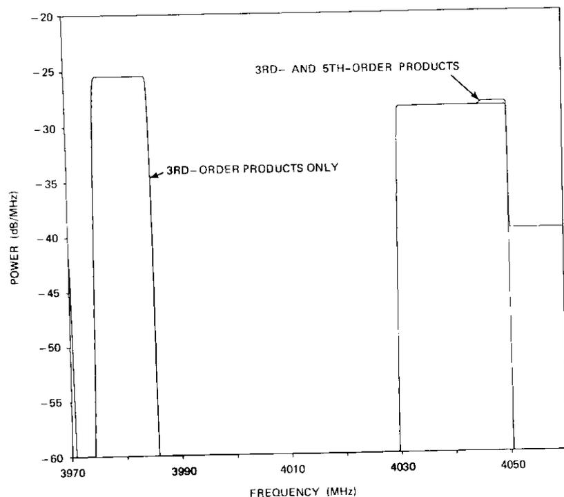
Figure 10. RF Intermodulation Power Spectral Density Generated by a Carrier with a Rectangular Spectrum and a Single Carrier
