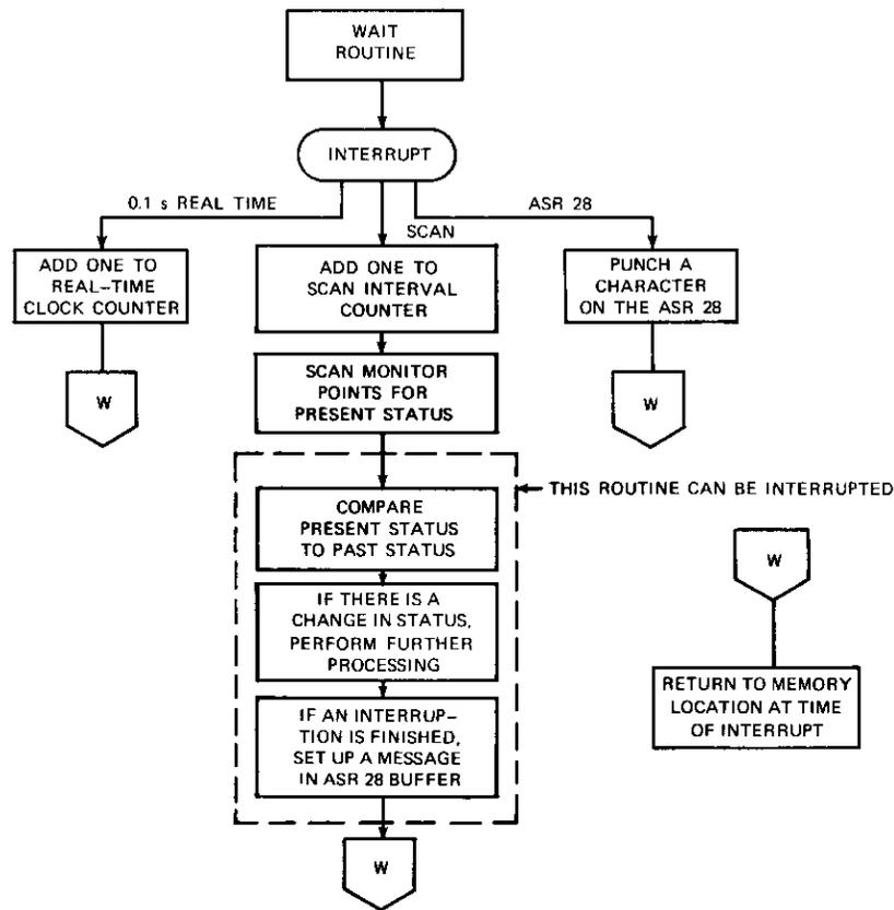
Figure 2. Block Diagram Description of Interruption Processing
