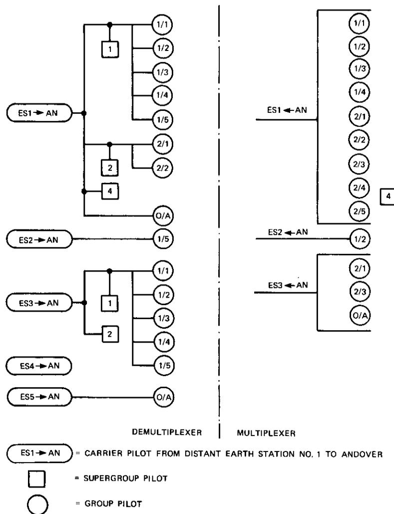
Figure 5. Topology of the Pilots Used for Evaluation of Data
