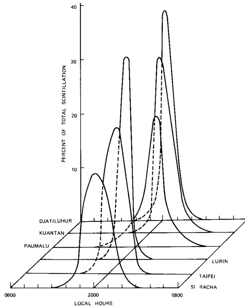
Figure 14. Diurnal Variation of Ionospheric Scintillation Greater than 0.5 dB at Djatiluhur, Kuantan, Paumalu, Lurin, Taipei, and Si Racha
