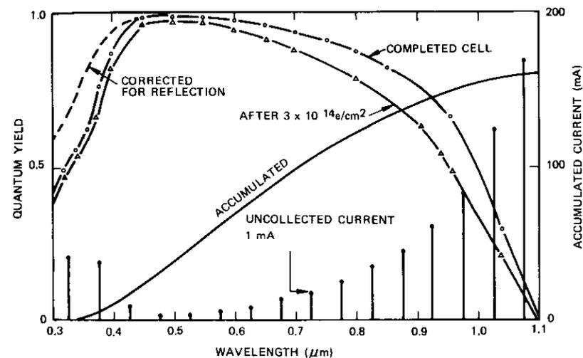
Figure 9. Quantum Yield of Typical Violet Cell Before and After Irradiation by  $3 \times 10^{14} \text{ e/cm}^2$  and Accumulated Cell Current and Current Lost per  $0.05 \mu\text{m}$  as Functions of Wavelength
