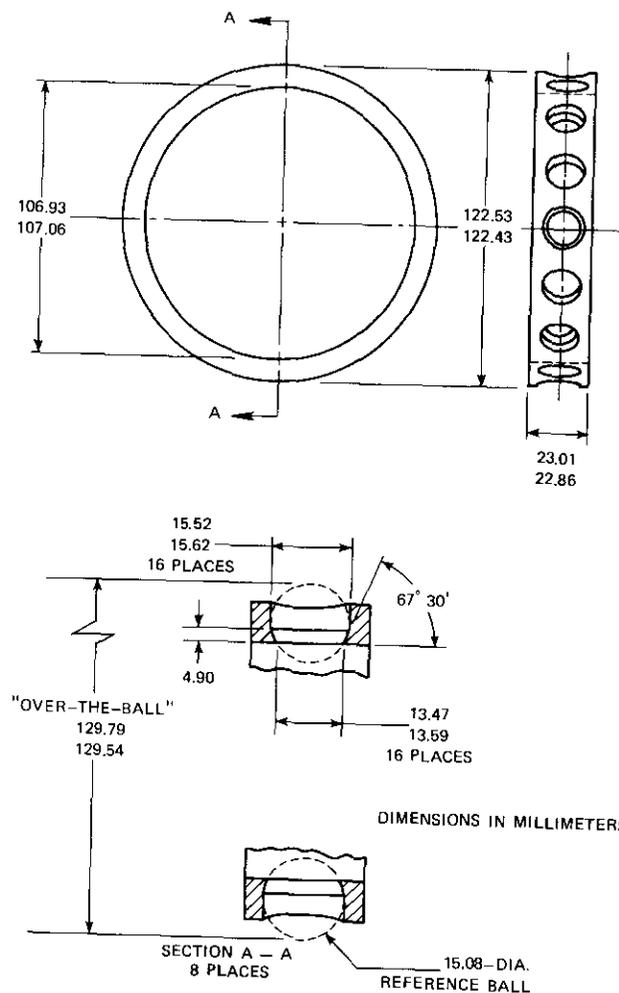
Figure 7. Flight Retainer
