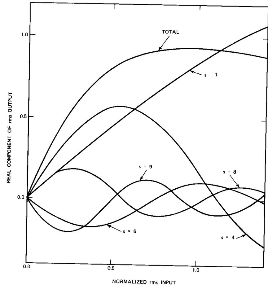
Figure 3. Bessel Function Expansion of the Real Component of the Single-Carrier Transfer Function
