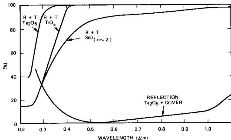
Figure 8. Reflection Plus Transmission for Three Oxides
