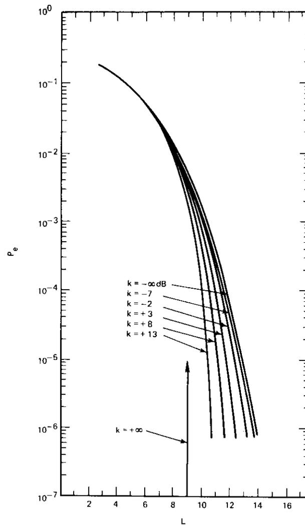
Figure 3d. Error Probabilities of 4-Phase PSK in the Presence of Gaussian Noise and Four Cochannel Interferences ( $H = 4, 4\phi$ )
