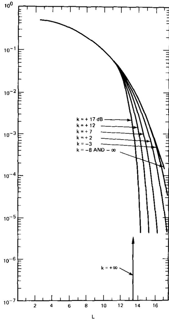
Figure 4c. Error Probabilities of 8-Phase PSK in the Presence of Gaussian Noise and Three Cochannel Interferences ( $H = 3, 8\phi$ )
