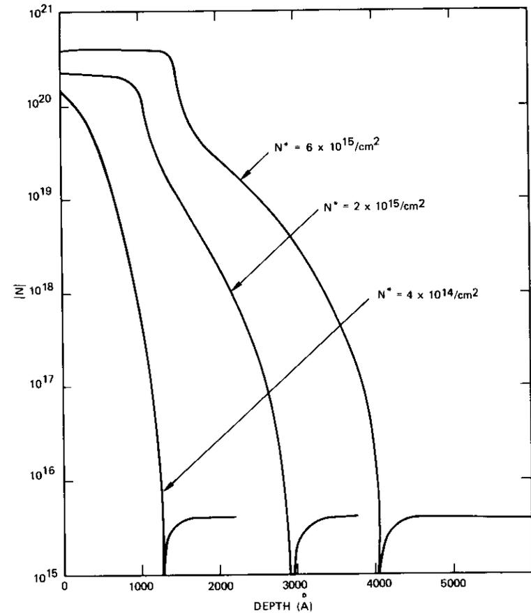
Figure 3. Diffusion Profiles for Phosphorus in Silicon for Three Junction Depths ( $N^*$  Denotes the Integrated Impurity Concentration)
