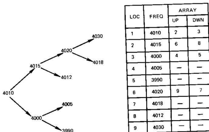
Figure 5. Tree Structure for Sorting Algorithm
