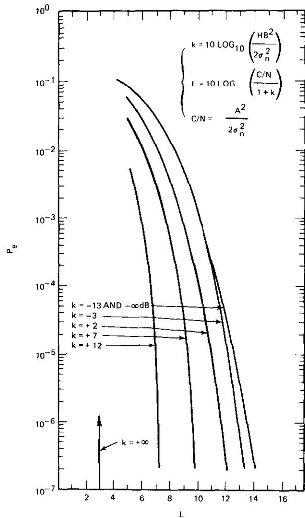
Figure 3a. Error Probabilities of 4-Phase PSK in the Presence of Gaussian Noise and One Cochannel Interference ( $H = 1, 4\phi$ )
