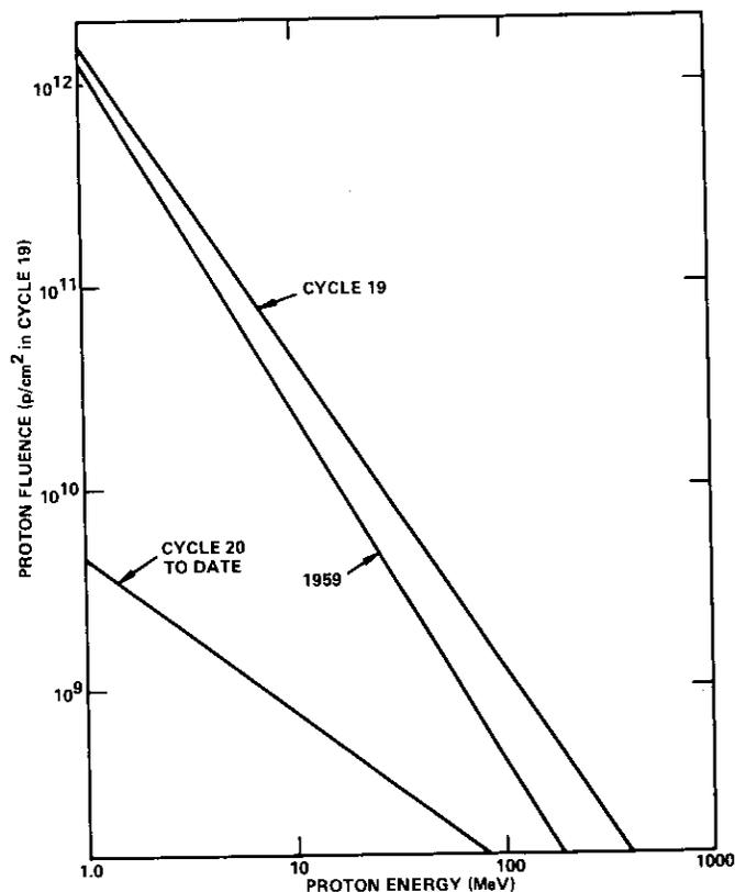
Figure 3. Unattenuated Solar Proton Fluence
