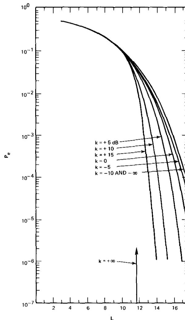
Figure 4b. Error Probabilities of 8-Phase PSK in the Presence of Gaussian Noise and Two Cochannel Interferences ( $H = 2, 8\phi$ )
