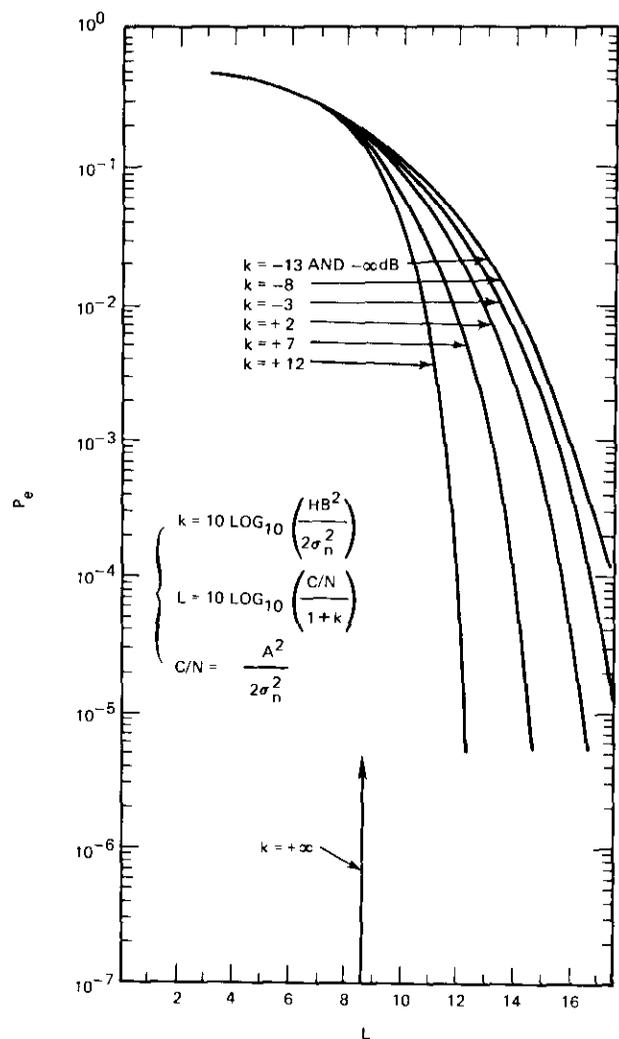
Figure 4a. Error Probabilities of 8-Phase PSK in the Presence of Gaussian Noise and One Cochannel Interference ( $H = 1, 8\phi$ )
