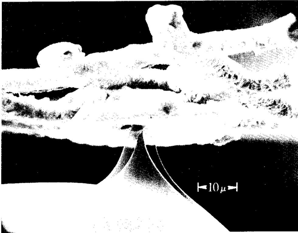
PLATE I. *Stereoscopic SE Image of a Germanium Tunnel Diode (side view)*
