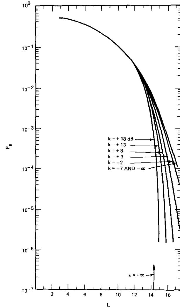
Figure 4d. Error Probabilities of 8-Phase PSK in the Presence of Gaussian Noise and Four Cochannel Interferences ( $H = 4, 8\phi$ )
