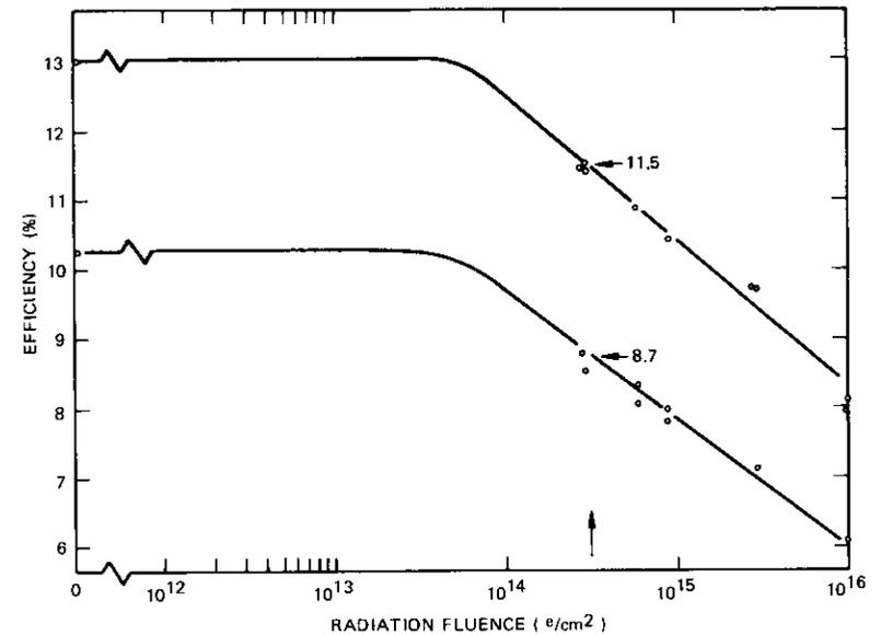
Figure 12. Violet Cell Compared with Commercial Cell for Radiation Damage with 1-MeV Electrons
