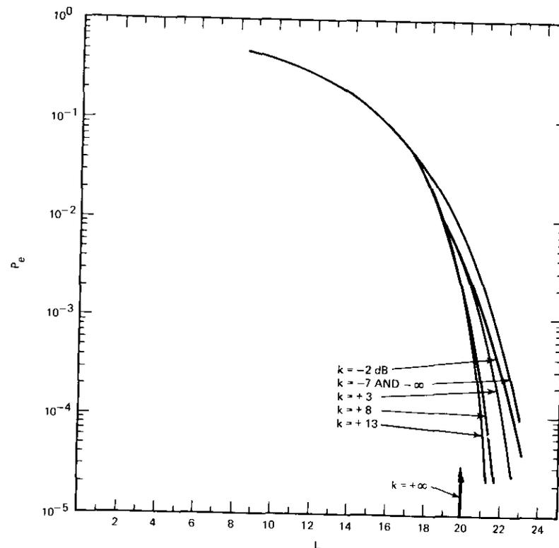
Figure 5d. Error Probabilities of 16-Phase PSK in the Presence of Gaussian Noise and Four Cochannel Interferences ( $H = 4, 16\phi$ )
