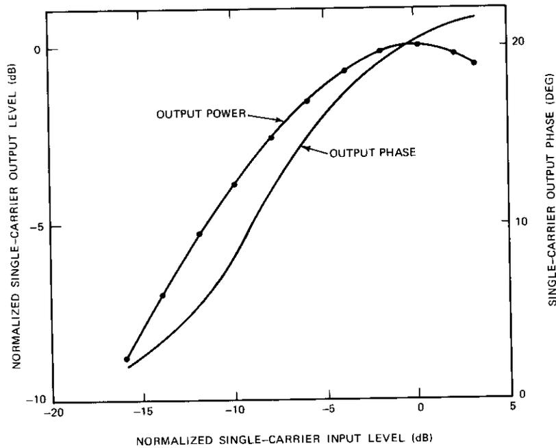
Figure 2. Measured Nonlinear Transfer Curves
