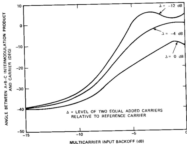
Figure 14. *Relative Phase Angle Between Intermodulation Product and Carrier vs Multicarrier Input Backoff*
