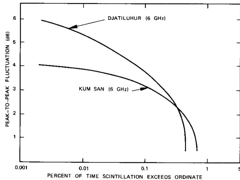
Figure 6. Cumulative Amplitude Distributions at Djatiluhur (6 GHz) and Kum San (6 GHz)
