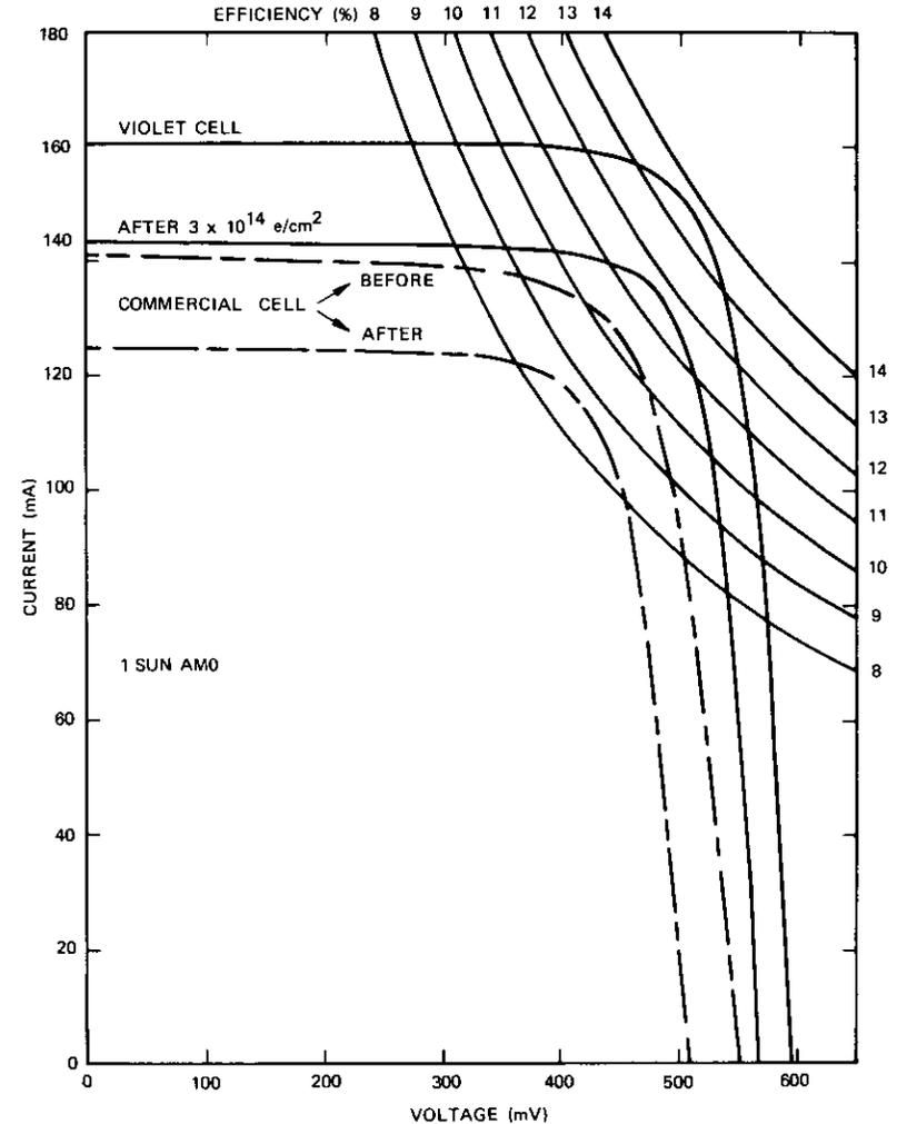
Figure 10. Typical I-V Curves for a Violet Cell and a Commercial Cell Before and After Irradiation by  $3 \times 10^{14} e/cm^2$
