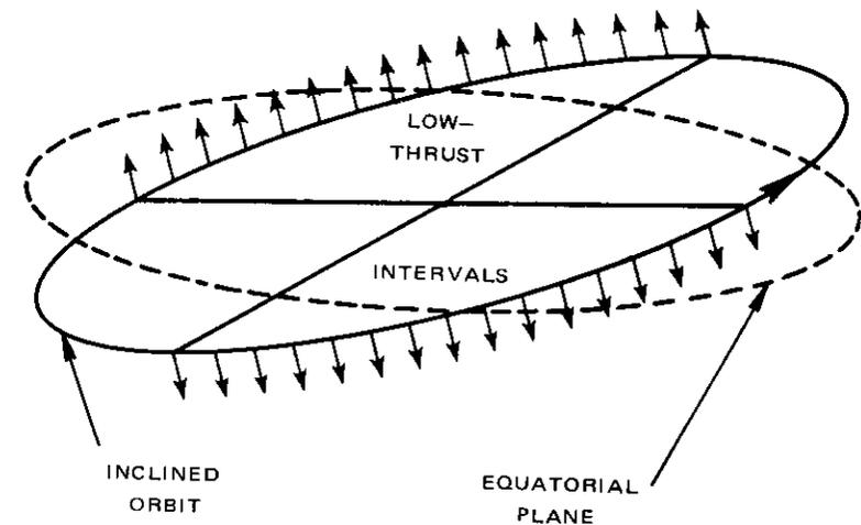
Figure 2. Thrust Program for North-South Stationkeeping with a Small Electric Thruster
