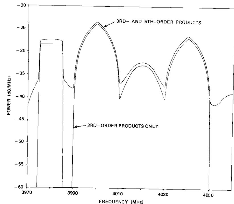
Figure 9. RF Intermodulation Power Spectral Density Generated by a Carrier Band and a Single Carrier
