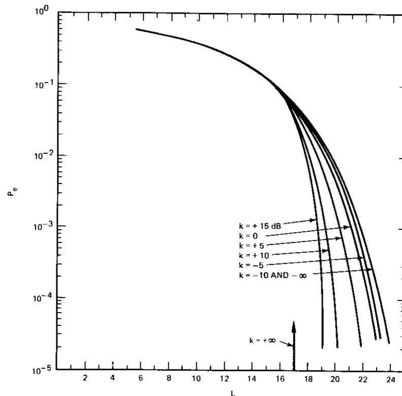
Figure 5b. Error Probabilities of 16-Phase PSK in the Presence of Gaussian Noise and Two Cochannel Interferences ( $H = 2, 16\phi$ )
