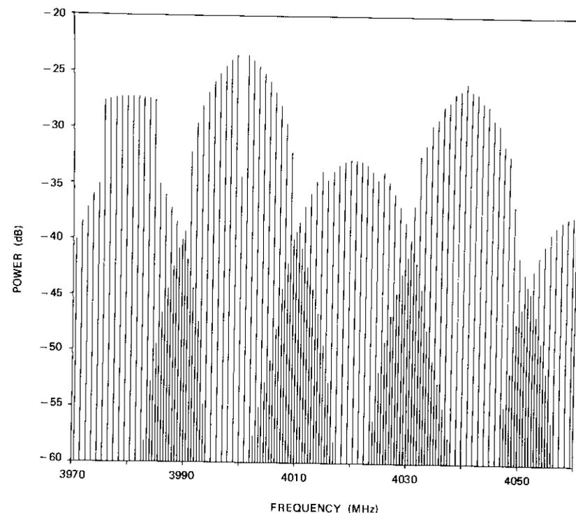
Figure 7. 3rd- and 5th-Order RF Intermodulation Products Generated by 10 Equal Carriers and a Single Carrier
