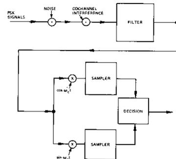
Figure 1. Receiving Scheme of PSK Systems
