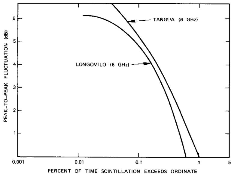
Figure 4. Cumulative Amplitude Distributions at Tangua (6 GHz) and Longovilo (6 GHz)
