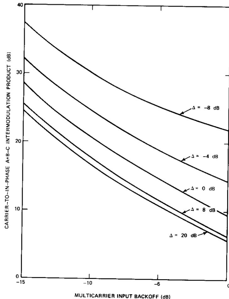
Figure 15. *Carrier-to-In-Phase Intermodulation Ratio vs Multicarrier Input Backoff*
