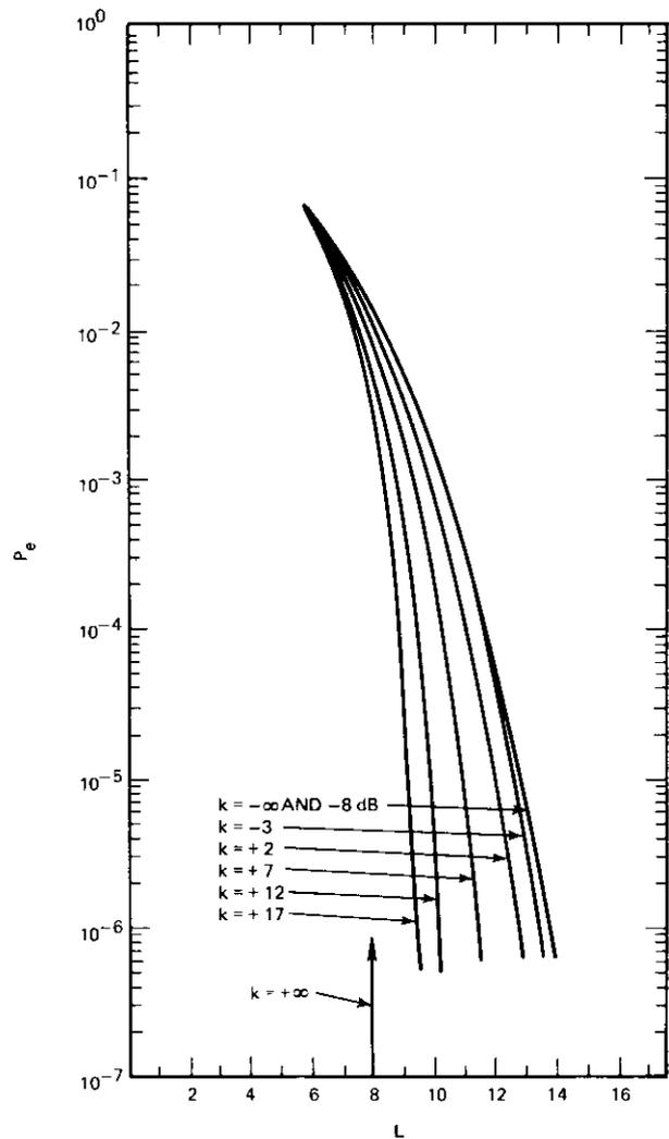
Figure 3c. Error Probabilities of 4-Phase PSK in the Presence of Gaussian Noise and Three Cochannel Interferences ( $H = 3, 4\phi$ )
