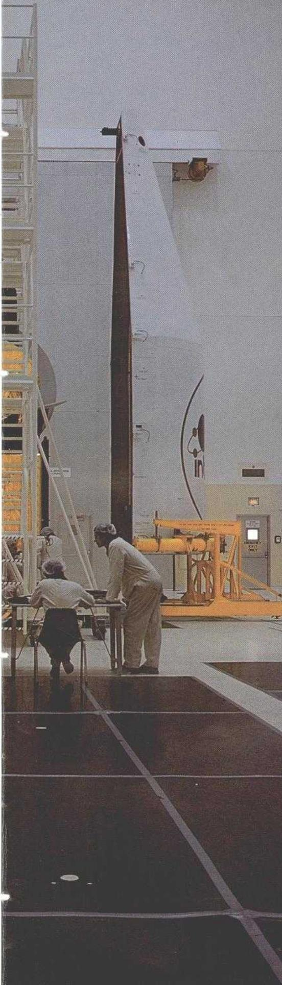
sulated spacecraft was slowly raised to the top of the launch vehicle and mated to the Centaur. The spacecraft was then turned on by a command from the Blockhouse and post-mate health of the spacecraft verified by technicians receiving the telemetry back at Building AO. L - 8 day was complete.
