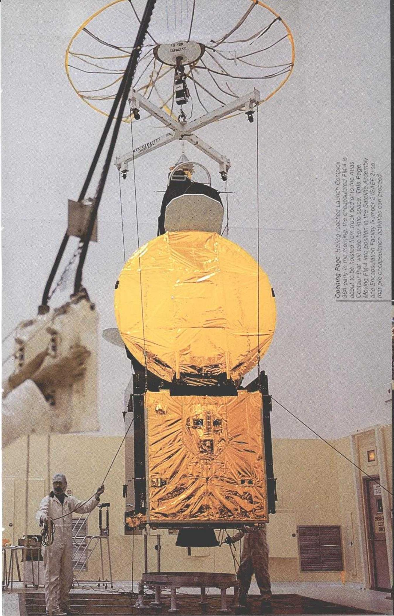
*Opening Page. Having reached Launch Complex 36A early in the morning, the encapsulated FM-4 is about to be hoisted from truck bed onto the Atlas Centaur that will take her into space. This Page Moving FM-4 into position in the Satellite Assembly and Encapsulation Facility Number 2 (SAEF-2) so that pre-encapsulation activities can proceed.*
