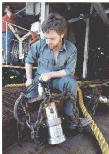
*Bottom Left, Vetter crewman with one of the air pressure guns used to generate underwater shock wave, a vital part of seismic work. Below Right, Small section of seismic vessel streamer cut open to reveal hydrophone.*
