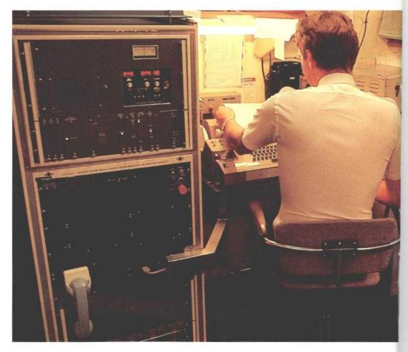
Radio officer on board Holiand America Cruises' S.S. Rotterdam using telex portion of ship's Mansat terminal.
