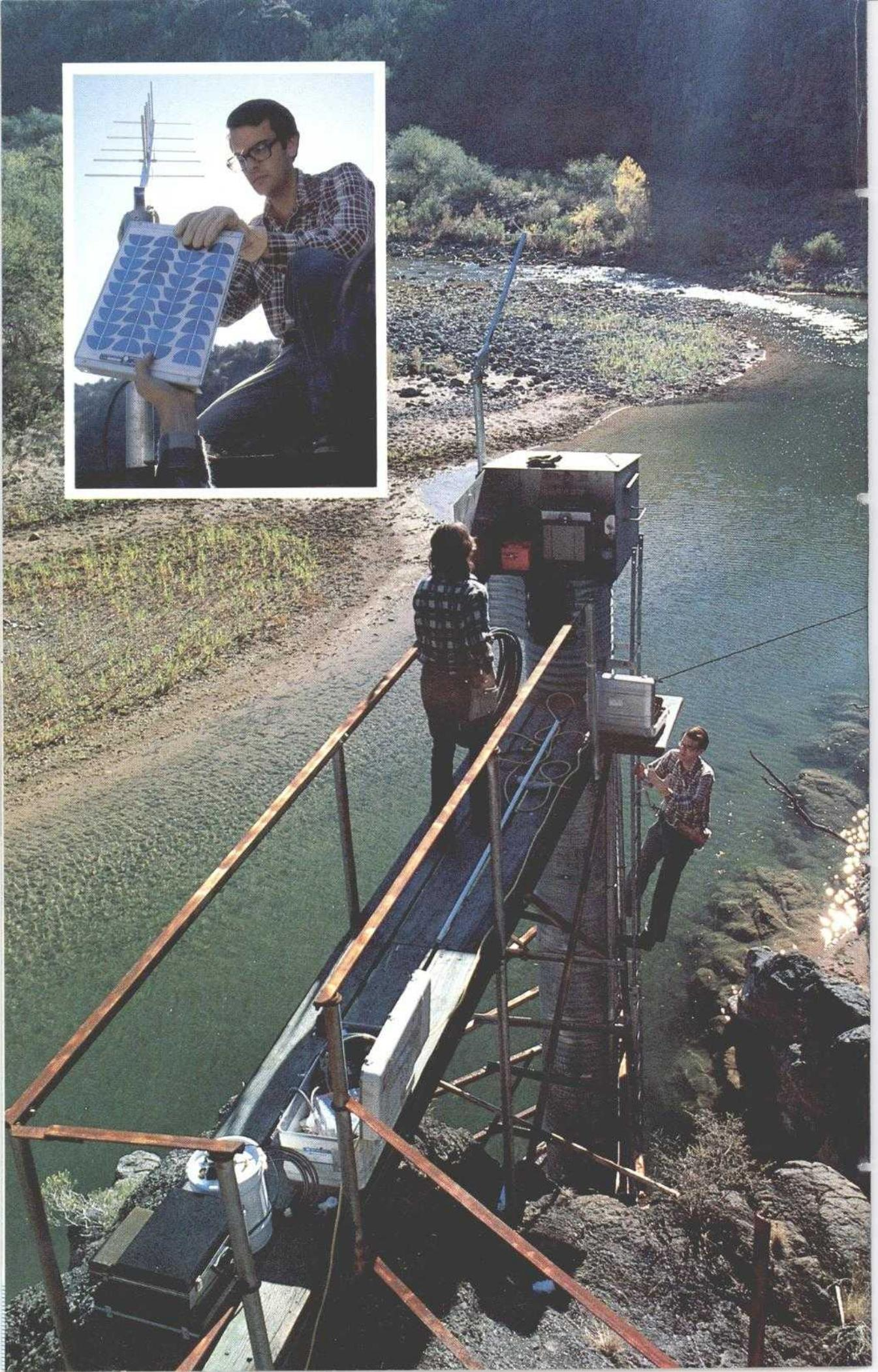
An employee of USGS or a co-operating organization hikes, takes four-wheel-drive vehicle or helicopter to the station, enters it, and either writes down the information shown or collects the paper tape from the water height recorder inside. After he reaches civilization, the data is then transmitted to Reston over phone lines.
