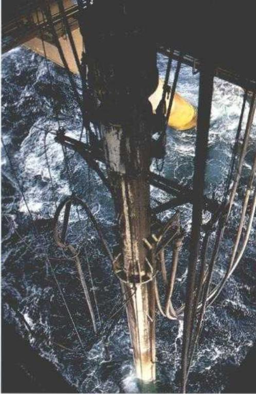
The drill stem enters water and penetrates the bottom of the sea floor. Inside the exterior conductor pipe is the surface casing and drill pipe leading down to the drill bit itself, chewing through layers of rock.
