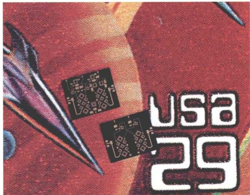
Two types of MMIC linearizers were designed for the solid-state power amplifier: The bottom chip is the version used in the C-band SSPA, while the top chip is used in an integrated amplifier. Both chips are pictured atop a 29¢ U.S. postage stamp.
