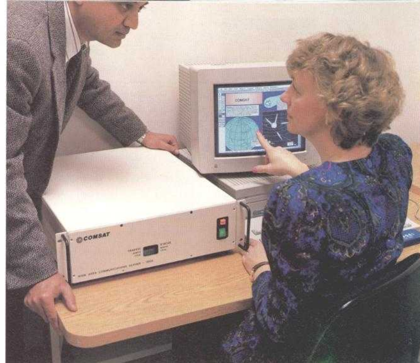
The NTD-developed wide area communications server provides NASA's Jet Propulsion Laboratory with efficient data communications over satellite links. The wide area server enables JPL to collect deep space data over satellites with data throughput comparable to those of fiber optic cables.
