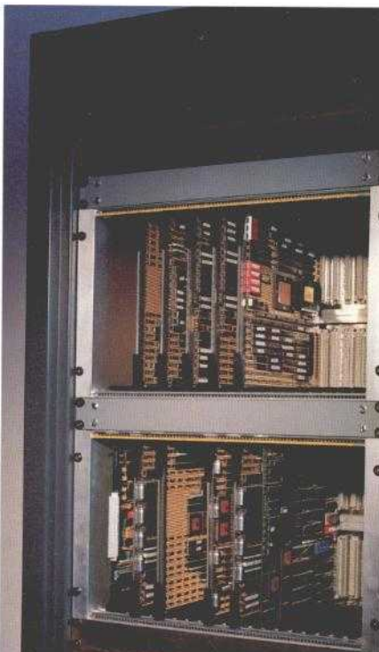
The NASA-sponsored HDTV codec uses subband filtering, along with SVQ. Subband filtering increases the compression ratio, decreases the compression hardware speed requirements and, in addition, makes available an enhanced NTSC channel.
