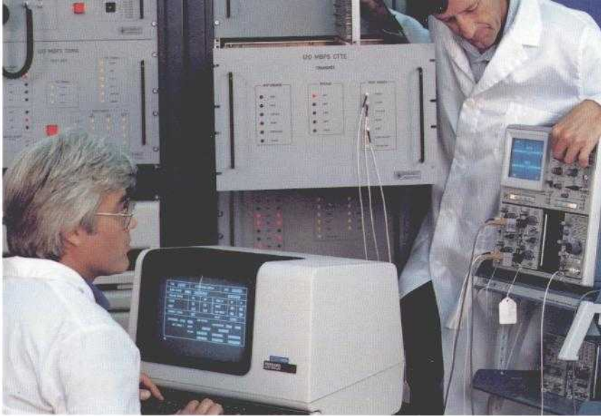
COMSAT Labs was the first to develop the INTELSAT 120-Mbit/s TDMA terminal in 1982. Here, NTD personnel complete the final checkout of the terminal.
