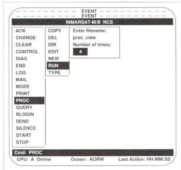
Figure 6. Inmarsat-M/B NCS menu selection screen facilitates the entry of operator commands
