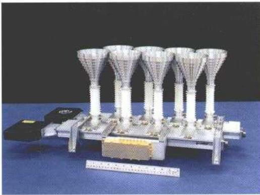
*The high polarization purity of the elements in the X-band array makes it suitable for dual-polarization applications.*
