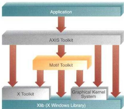
*The AXIS Toolkit design uses the layered approach found in the X Window System and Motif. The design architecture builds on the functionality found in X Window and Motif and provides extended capabilities that offer the software developer the most flexible system possible.*
