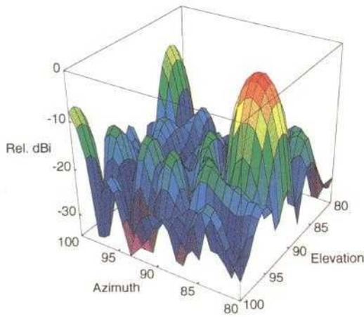
*Testing of the Ku-band active phased array included measuring radiation patterns at multiple frequencies and power levels, performing holographic measurements, and evaluating system performance of intermodulation levels and bit error ratios under multicarrier conditions.*
