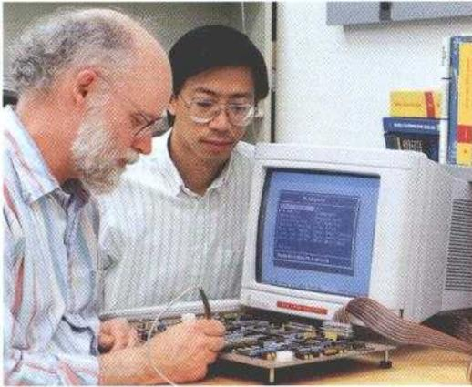
Two CTD engineers test the modulator for the programmable digital modem being developed for NASA. The modulator operates over the full data rate range without any component changes or filter bandwidth switching.
