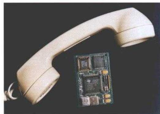
*The COMSAT 1,200-bit/s LSF-Split VQ voice codec has been optimized to run on a miniature digital signal processing platform, enabling it to be used in a variety of voice telephony, digital radio, and voice messaging applications.*
