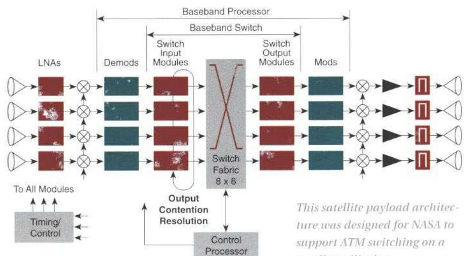
This satellite payload architecture was designed for NASA to support ATM switching on a small satellite bus.
