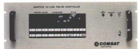
*The prototype ULPC system was built to test and validate the design features of a complete user interface and remote control capability.*
