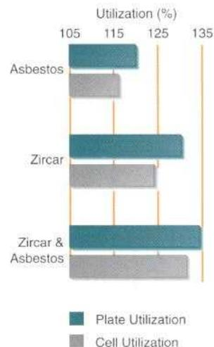
*Destructive physical analysis of Ni-H<sub>2</sub> cells indicates that the coefficient of positive plate active material utilization is higher in cells containing two layers of Zircar™, or one layer of Zircar™ and one layer of fuel-cell-grade asbestos, compared to cells with one layer of asbestos.*
