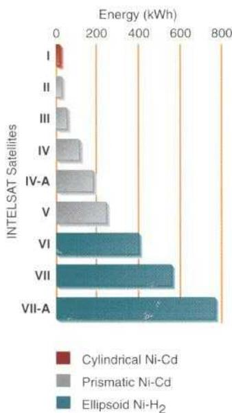
Battery capacity has increased significantly from generation to generation of communications satellites.
