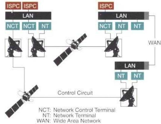
*The ISPC provides comprehensive system planning and network management capabilities for networks of universal modems (operating either as NTs or NCTs) on DSCS, SKYNET, SYRACUSE, and NATO satellites.*
