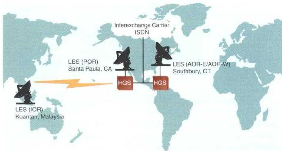
*The high-data-rate gateway switch enables CMC to provide switched 56/64-kbit/s services to mobile users throughout the world.*
