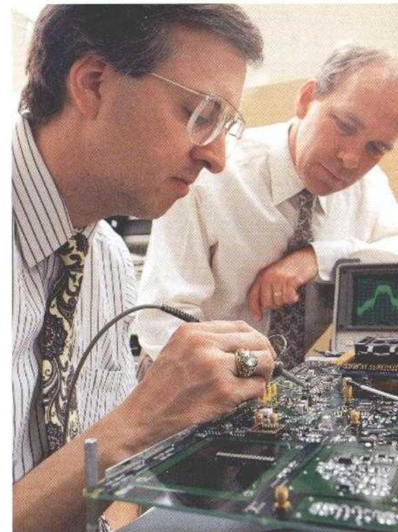
CTD engineers test the MSP-10 in a board designed for use in intermediate data rate systems. The board contains all the functions for both transmit and receive, with fully synthesized IF channelization. In addition to modem functions, the card contains a Viterbi decoder chip for rate 1/2 and 3/4 operation.
